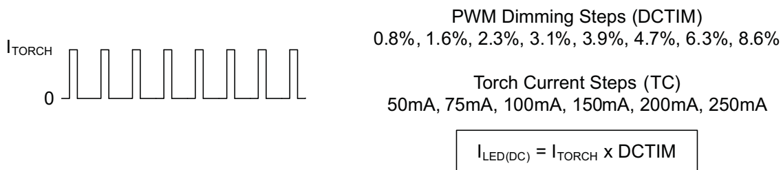
Figure 39. PWM Dimming Principle
