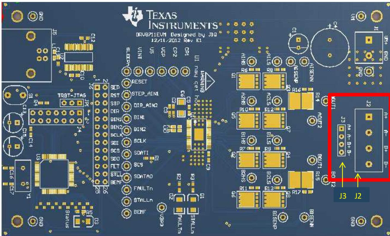
Figure 3. Motor Outputs
