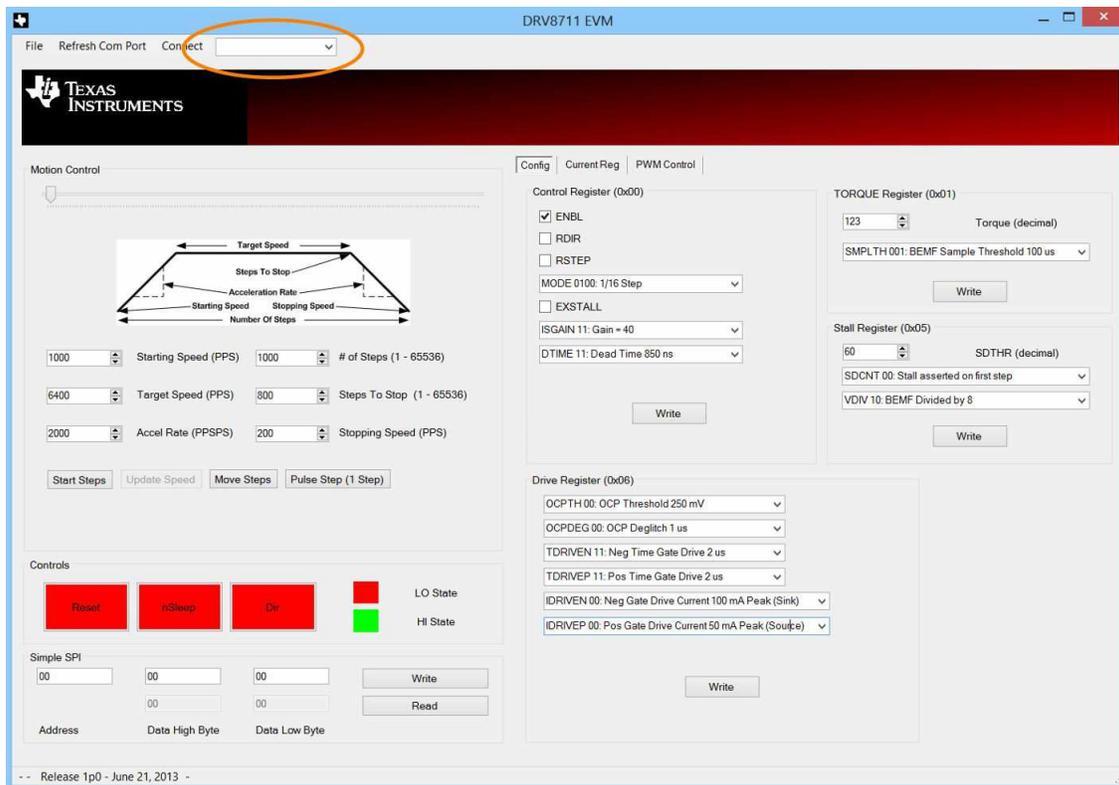
7. All defaults have been preset for a 16-step operation using the supplied motor. Click the four write buttons on the Config page as shown below.
