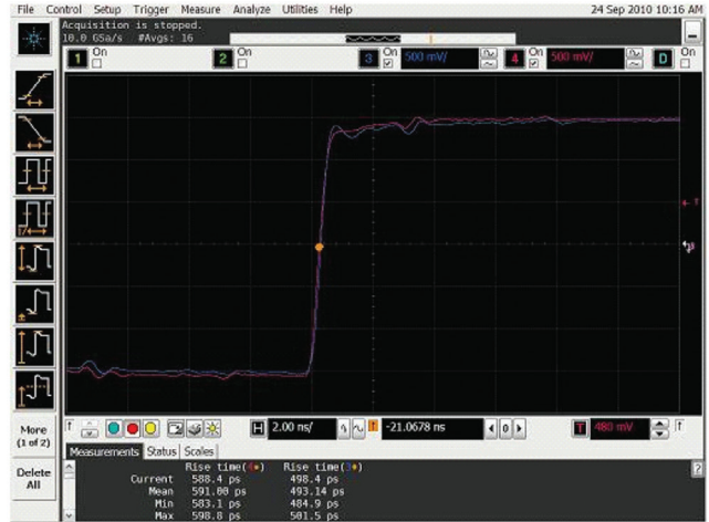
Time domain step response of N2796A (with Agilent MSO9404A)
