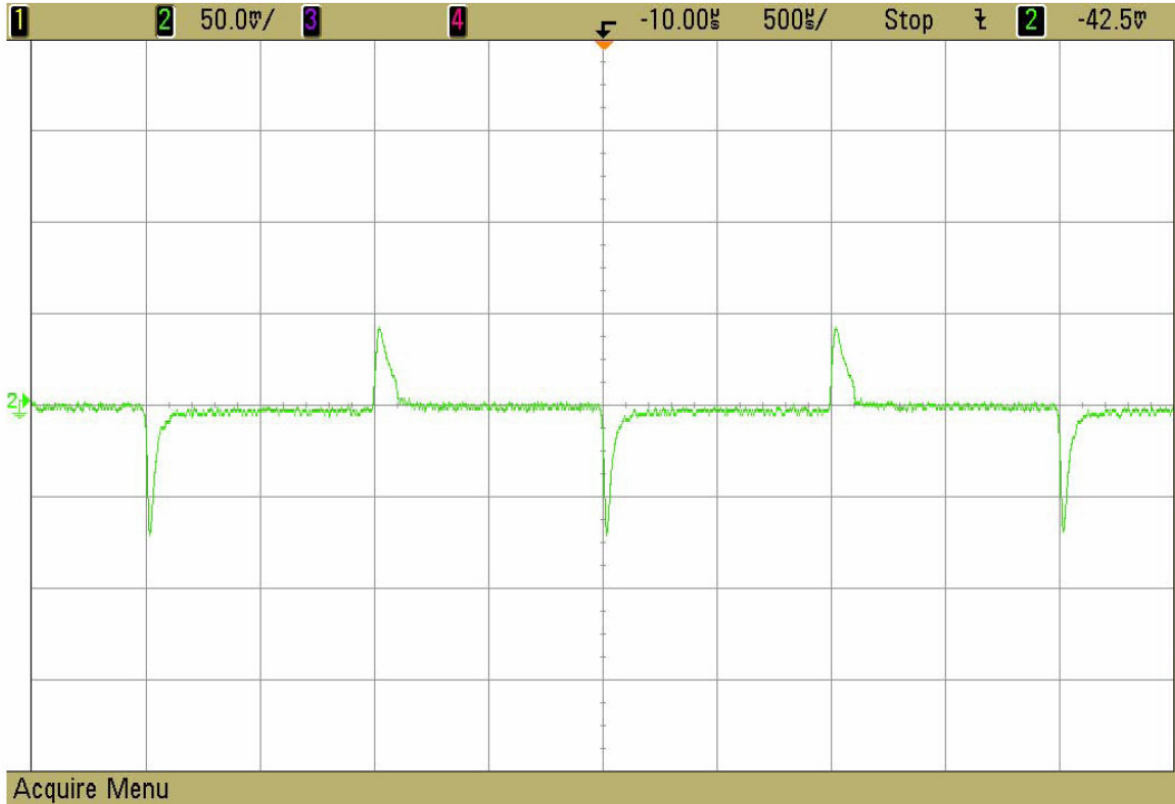
Figure 4. Transient Response Waveform at 4.2Vin and 0.75 - 1.5Aout – 500uS and 50mV / div
