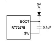
Figure 2. External Bootstrap Diode
