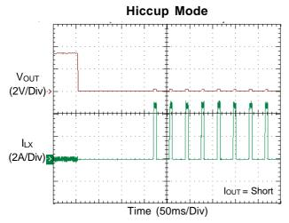
Figure 5. Hiccup Mode Under Voltage Protection
