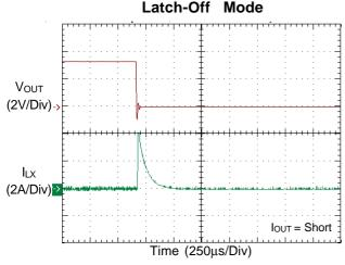
Figure 6. Latch-Off Mode Under Voltage Protection
