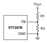
Figure 1. Output Voltage Setting
