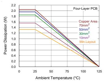
Figure 8. Derating Curve of Maximum Power Dissipation
