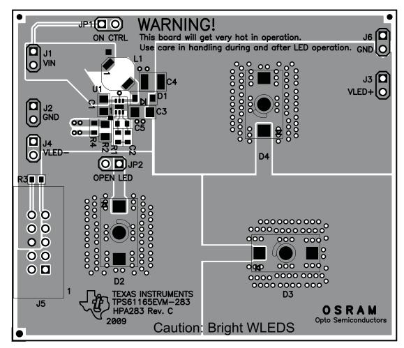
Figure 4. Assembly Layer
