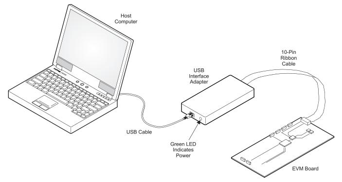
Figure 1. USB Interface Adapter Quick Connection Diagram
