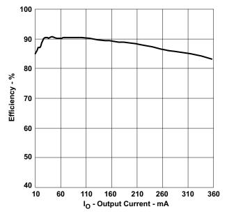
Figure 3. LED Efficiency vs Output Current
