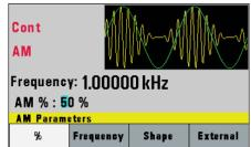
Both models provide AM and FM modulation along with linear/logarithmic sweep and built-in counter capabilities. Internal and external sources can be used for triggering and modulating the signal.
