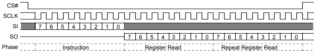
Figure 10.6 Read Configuration Register (RDCR) Command Sequence
