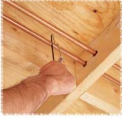
Will reach into tight spaces where standard hacksaw frames cannot fit to make a cut.
