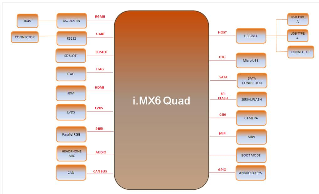
Figure 1-1 Functional Block Diagram of SABRE Lite Board
