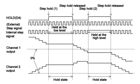
When the hold bit in the serial data, D4 (100, \*, D4, \*\*\*), is set to 1, the external step state at that time is held without change as the internal step state.
