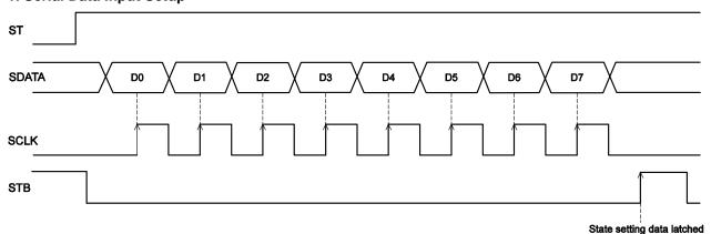
First set STB low and then input the SDATA and SCLK signals. The SCLK signal is not accepted when STB is high. SDATA inputs the data in the order D0, D1, ... D6, D7.
