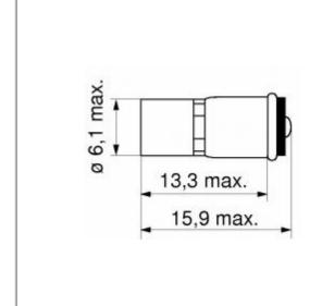
Part Number: 1510145UR3 Serial Number: 15101 Based LED type: StarLED Size (inch): T-1 3/4 Size (mm): T6
