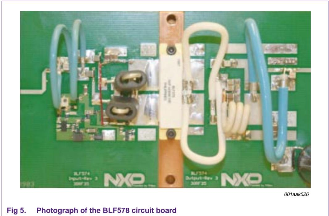
Fig 5. Photograph of the BLF578 circuit board
