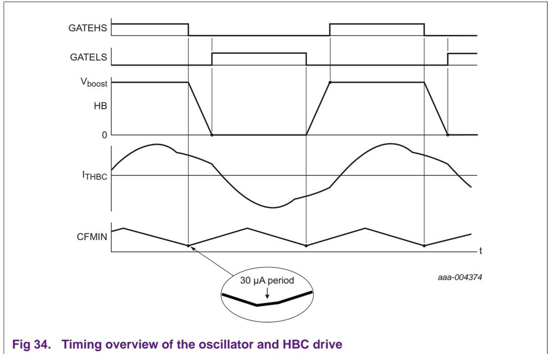
Fig 34. Timing overview of the oscillator and HBC drive
