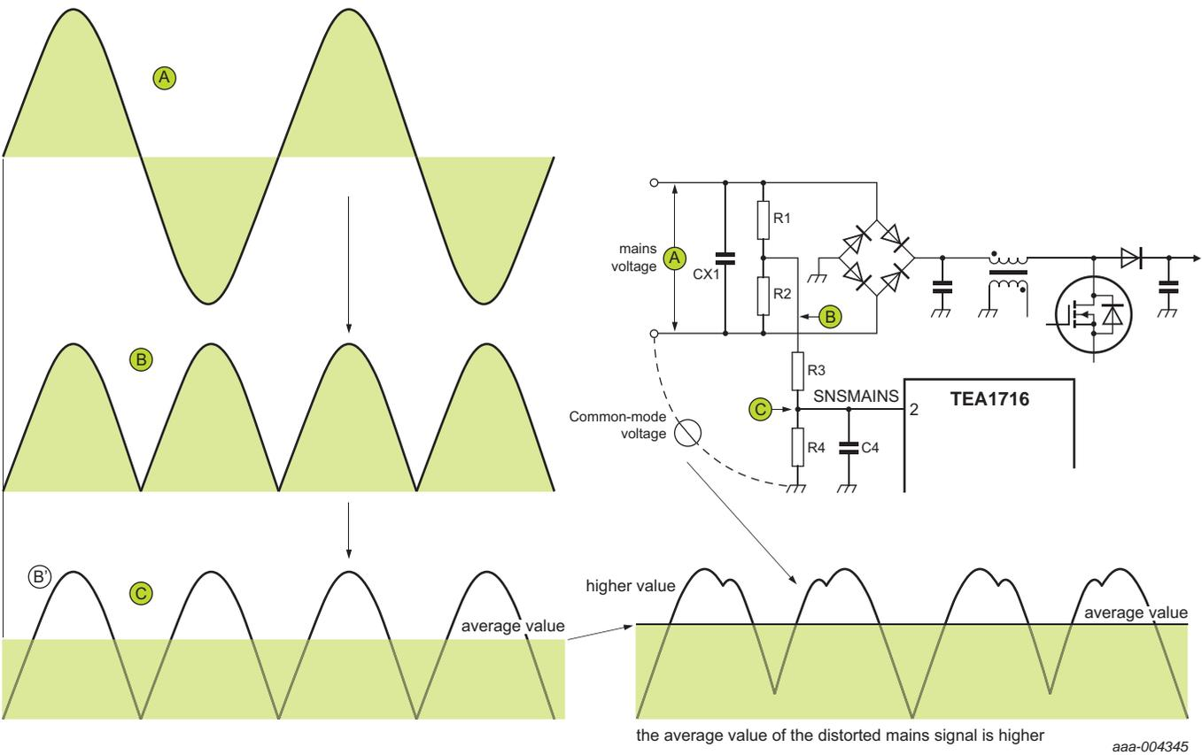
Fig 25. Higher SNSMAINS value because of measured signal distortion
