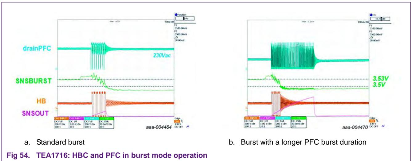
Fig 54. TEA1716: HBC and PFC in burst mode operation
