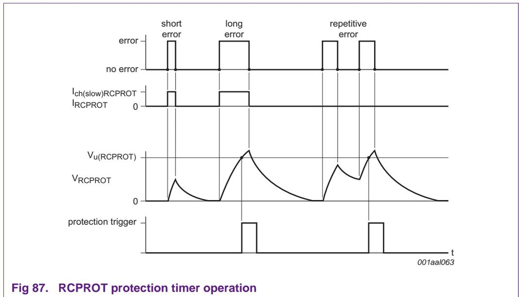
Fig 87. RCPROT protection timer operation
