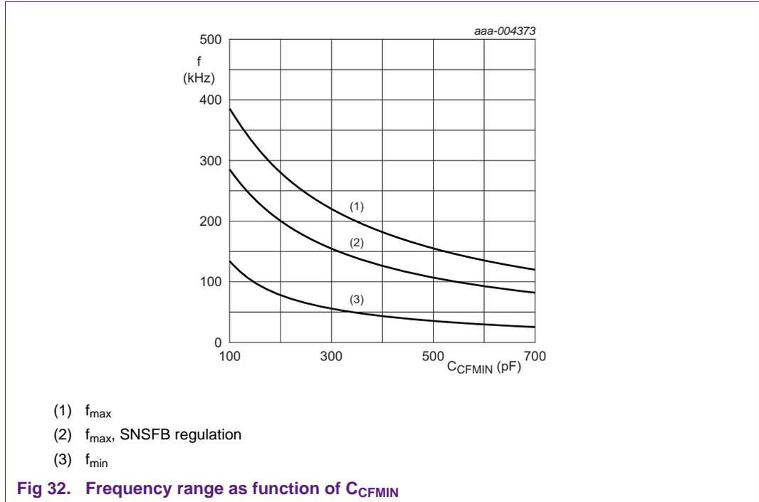
The oscillator frequency depends on the charge and discharge current of the capacitor on the CFMIN pin. The charge and discharge current consists of a fixed part which determines the minimum frequency and the SNSFB and SSHBC/EN pins control functions drive a variable part.
