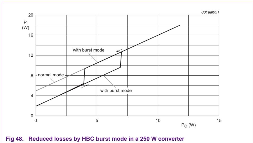
Fig 48. Reduced losses by HBC burst mode in a 250 W converter
