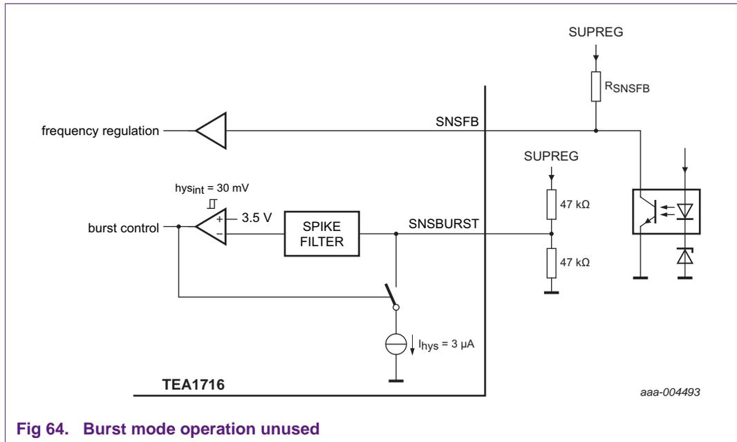
Fig 64. Burst mode operation unused
