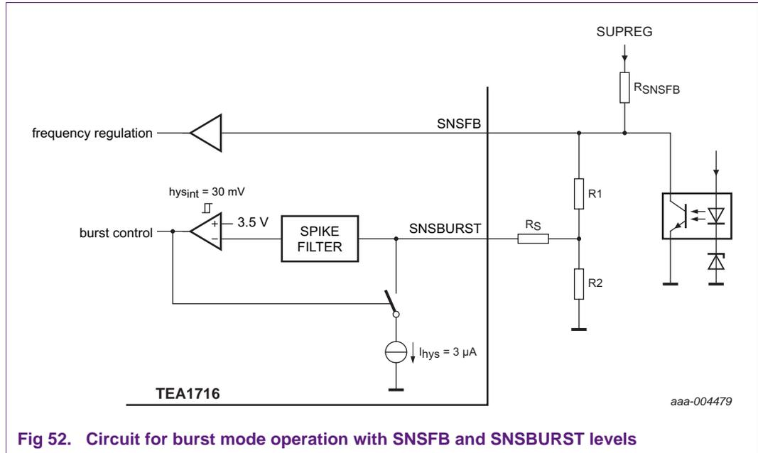
Fig 52. Circuit for burst mode operation with SNSFB and SNSBURST levels
