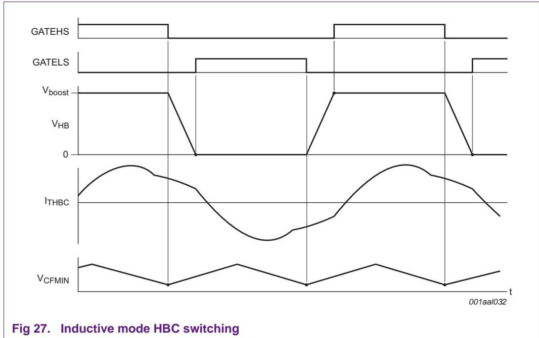
Fig 27. Inductive mode HBC switching
