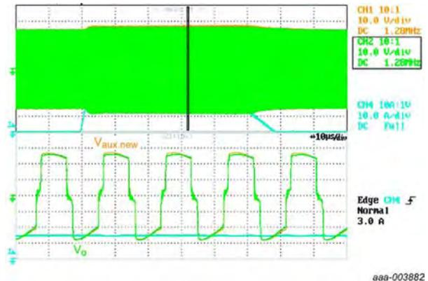
b. Correct coupling  $V_{aux(new)}$  to  $V_{out}$  at high output current
