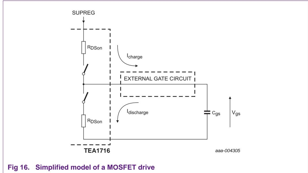
Fig 16. Simplified model of a MOSFET drive
