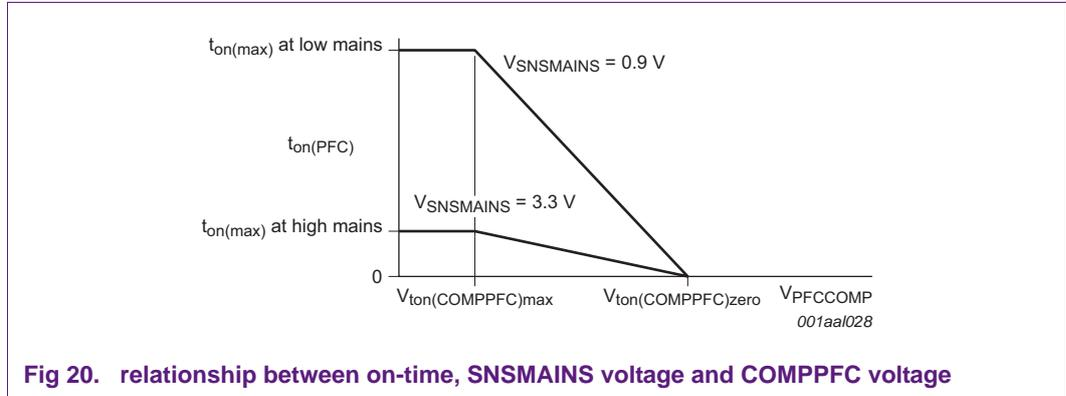
Fig 20. relationship between on-time, SNSMAINS voltage and COMPFC voltage
