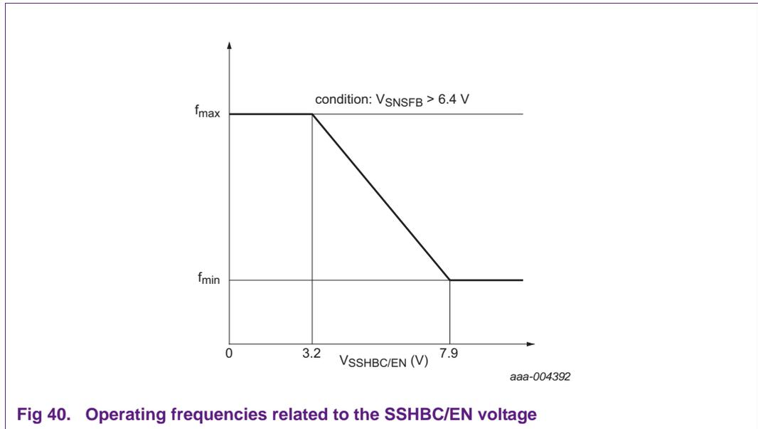
Fig 40. Operating frequencies related to the SSHBC/EN voltage
