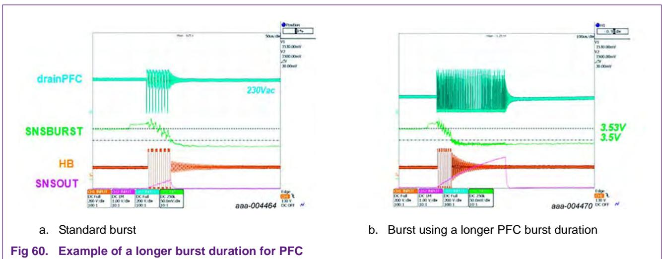
10.8.1 Alternating between burst and normal operation
