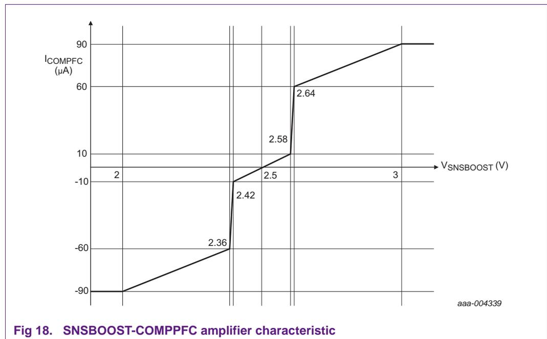
**Fig 18. SNSBOOST-COMPPFC amplifier characteristic**
