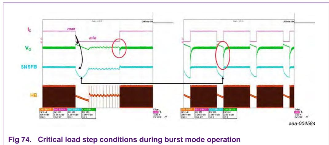
Fig 74. Critical load step conditions during burst mode operation
