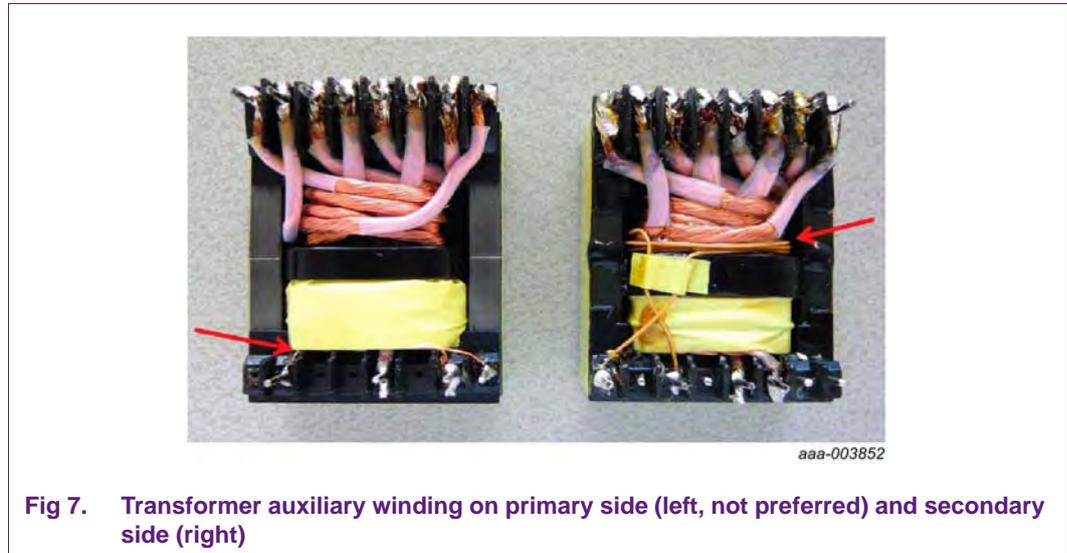
**Fig 7. Transformer auxiliary winding on primary side (left, not preferred) and secondary side (right)**
