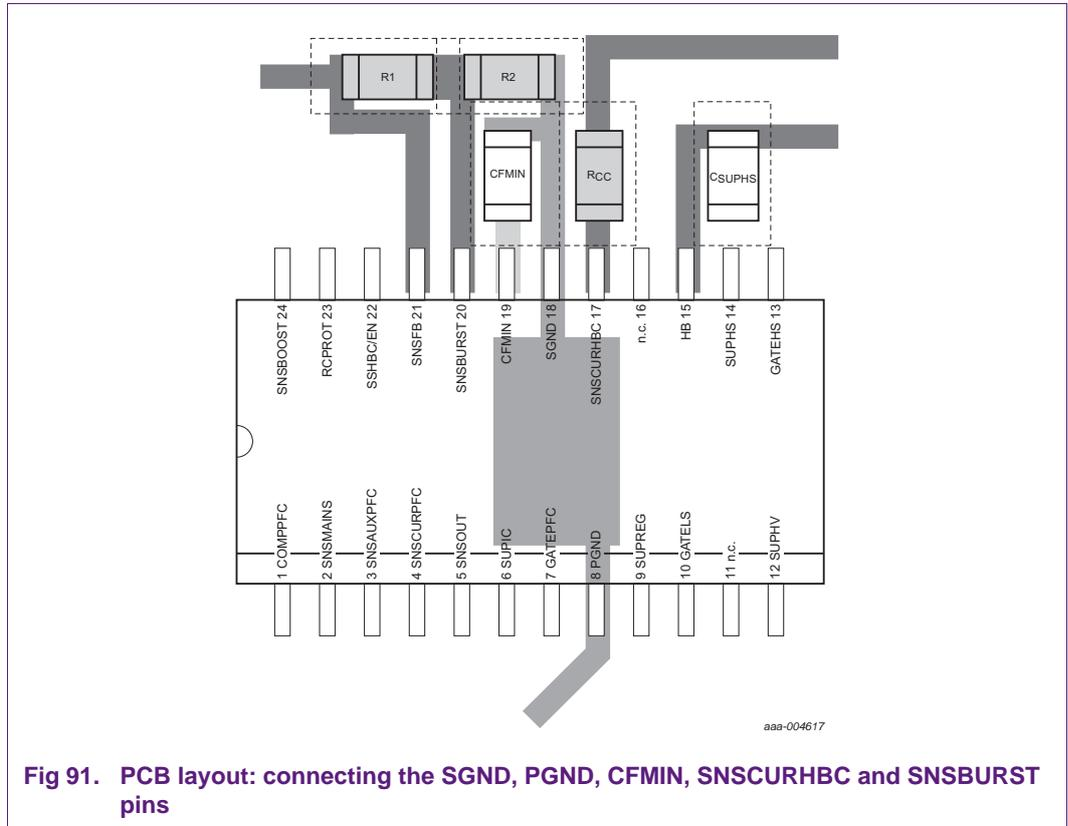
Fig 91. PCB layout: connecting the SGND, PGND, CFMIN, SNSCURHBC and SNSBURST pins
