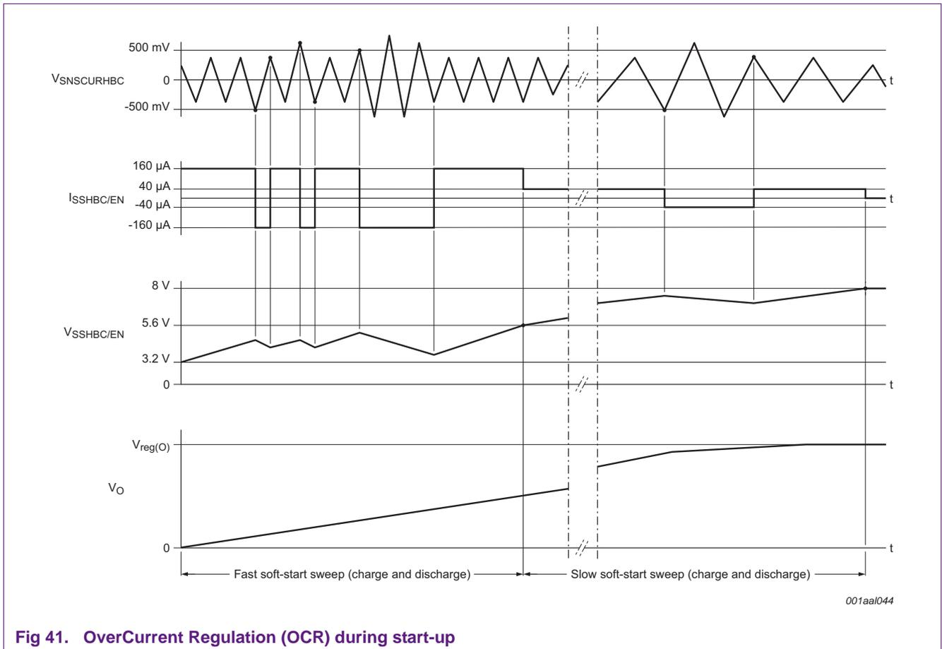
Fig 41. OverCurrent Regulation (OCR) during start-up
