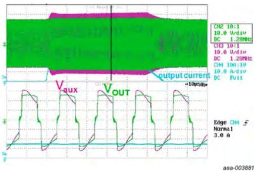
a. Bad coupling  $V_{aux}$  to  $V_{out}$  at high output current
