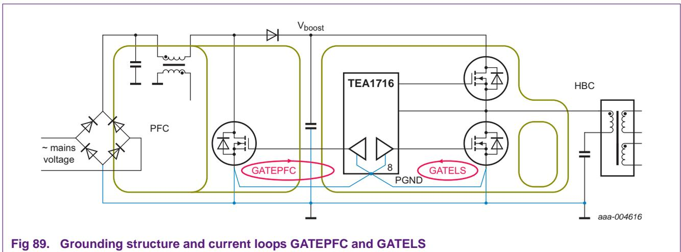
Fig 89. Grounding structure and current loops GATEPFC and GATELS
