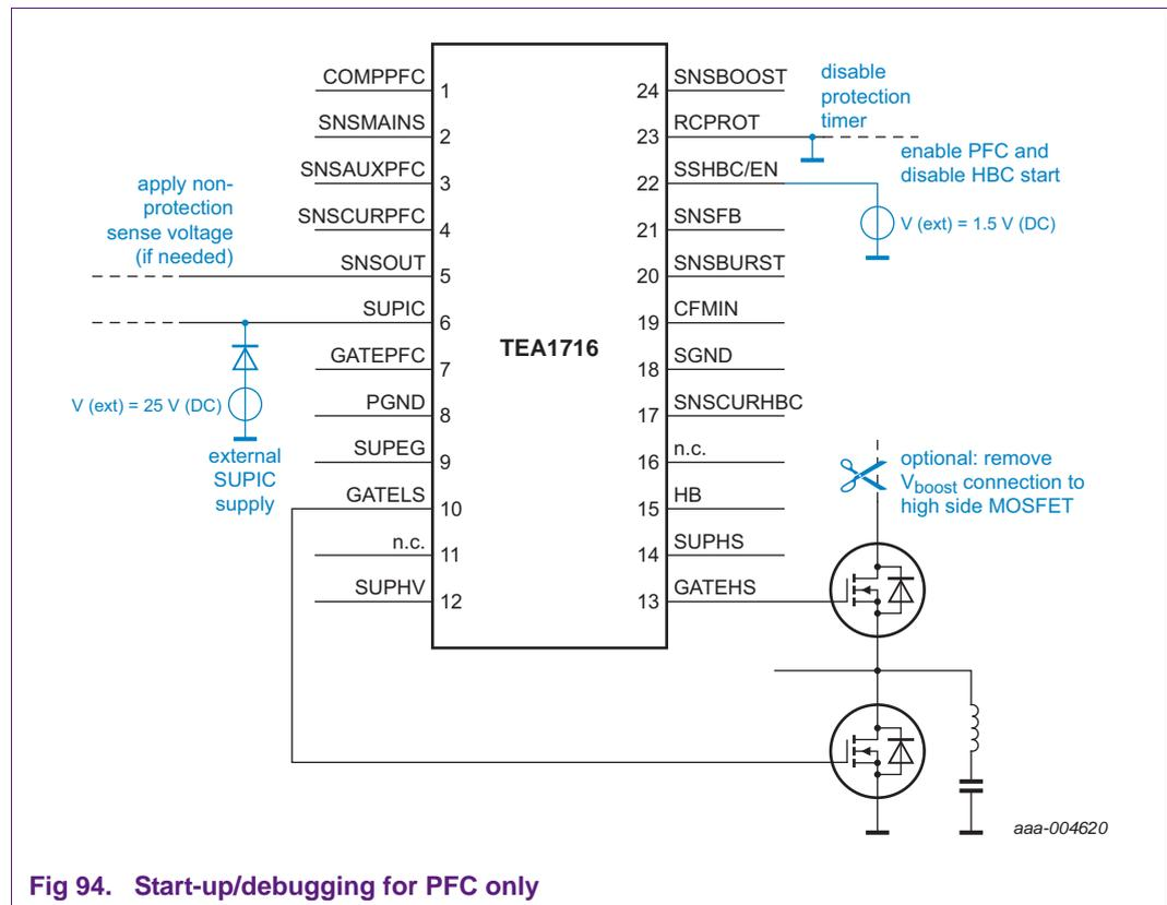
Fig 94. Start-up/debugging for PFC only
