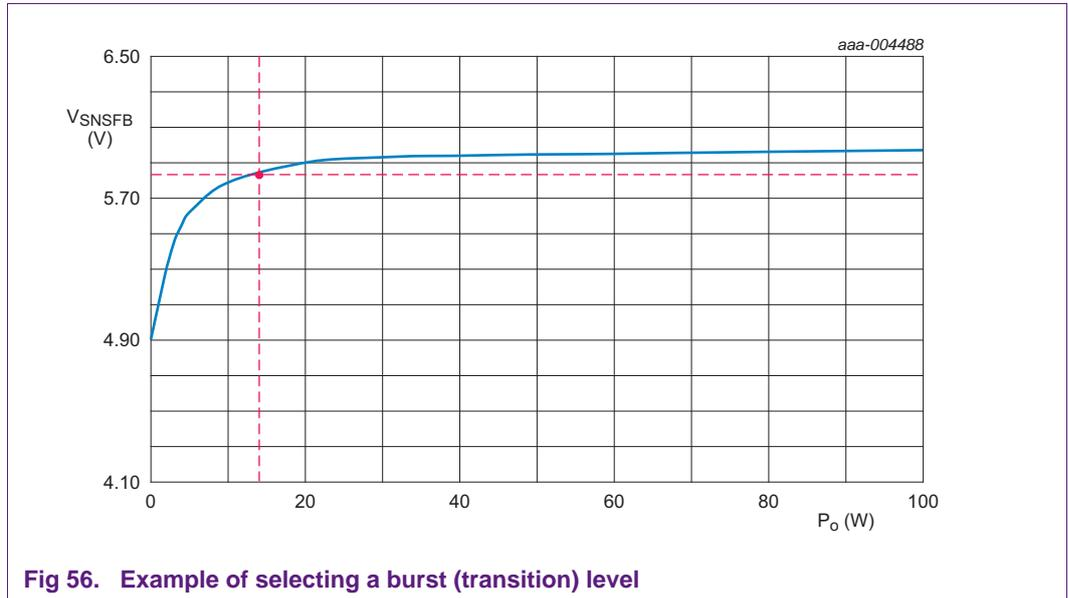
Fig 56. Example of selecting a burst (transition) level
