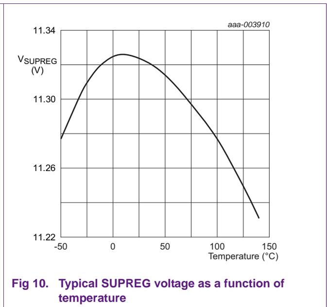
Fig 10. Typical SUPREG voltage as a function of temperature
