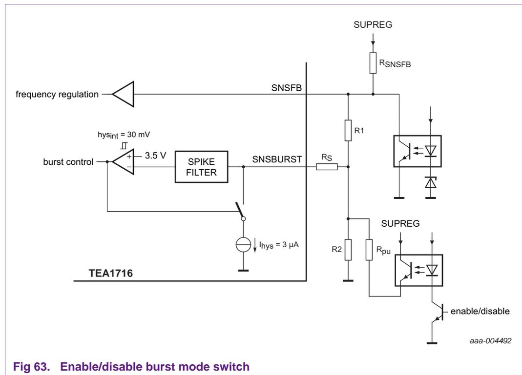
**Fig 63. Enable/disable burst mode switch**
