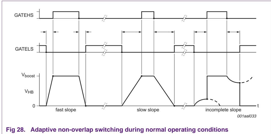
**Fig 28. Adaptive non-overlap switching during normal operating conditions**
