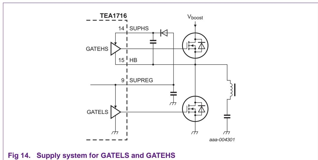
Fig 14. Supply system for GATELS and GATEHS
