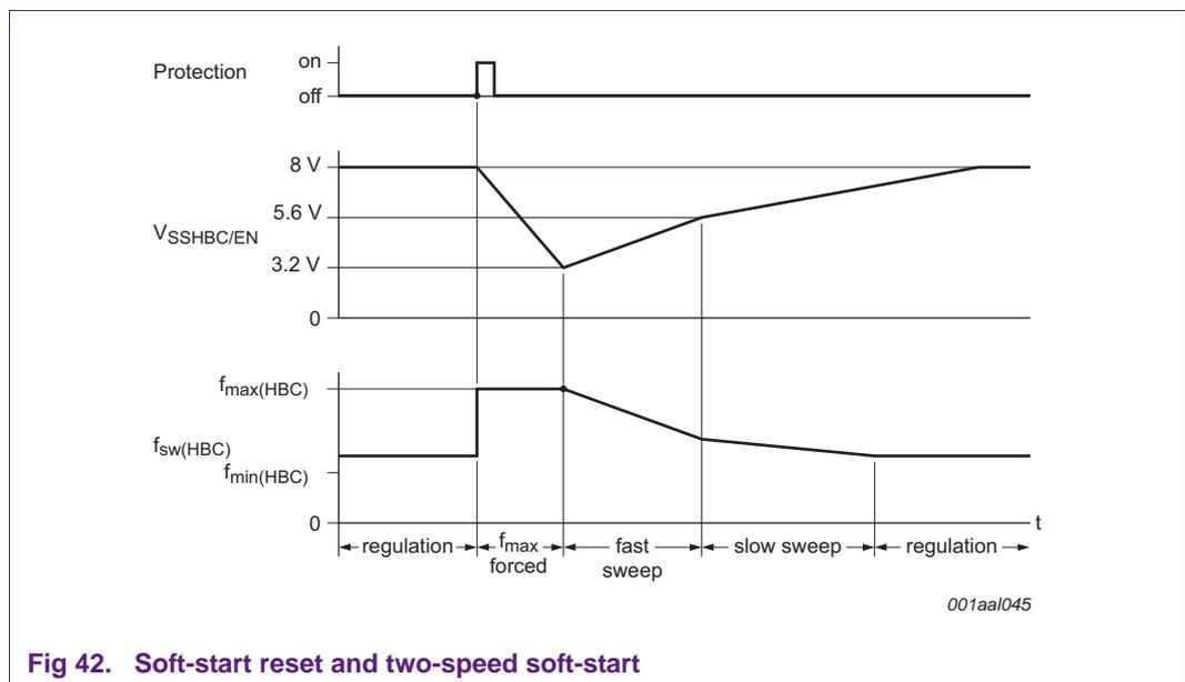
Fig 42. Soft-start reset and two-speed soft-start
