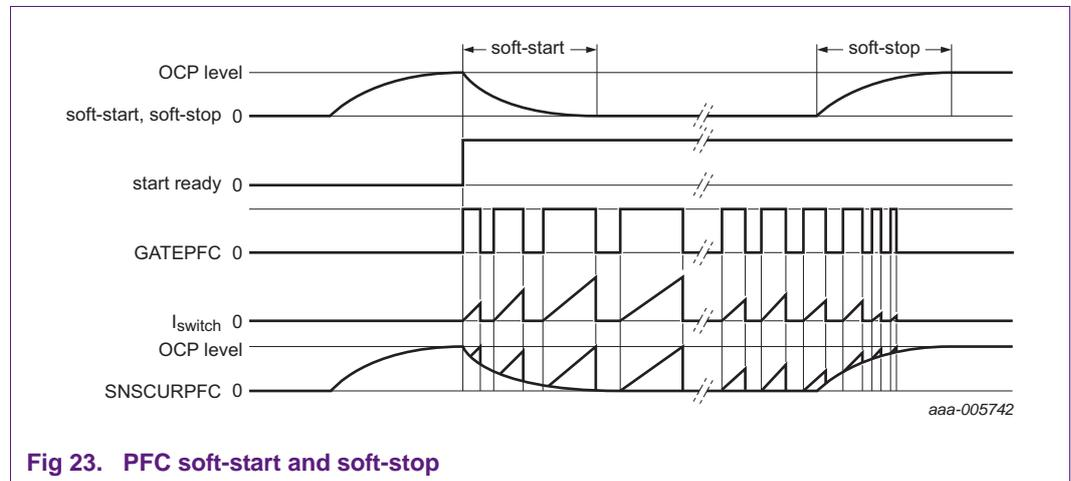
**Fig 23. PFC soft-start and soft-stop**
