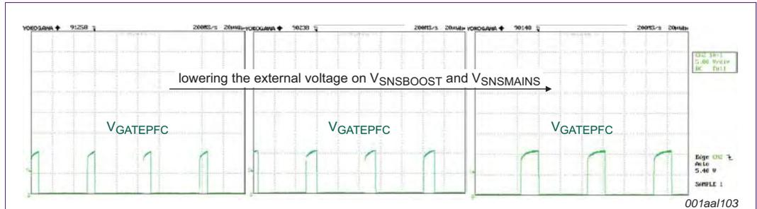
Fig 95. Typical GATEPFC signals without mains voltage
