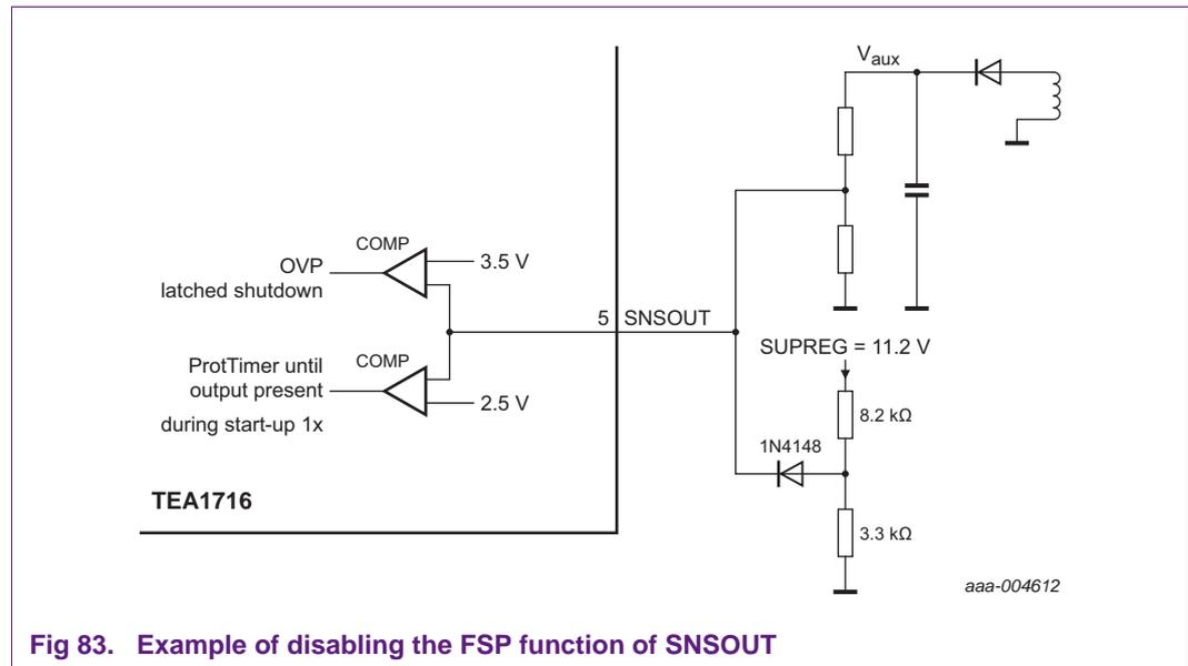
**Fig 83. Example of disabling the FSP function of SNSOUT**
