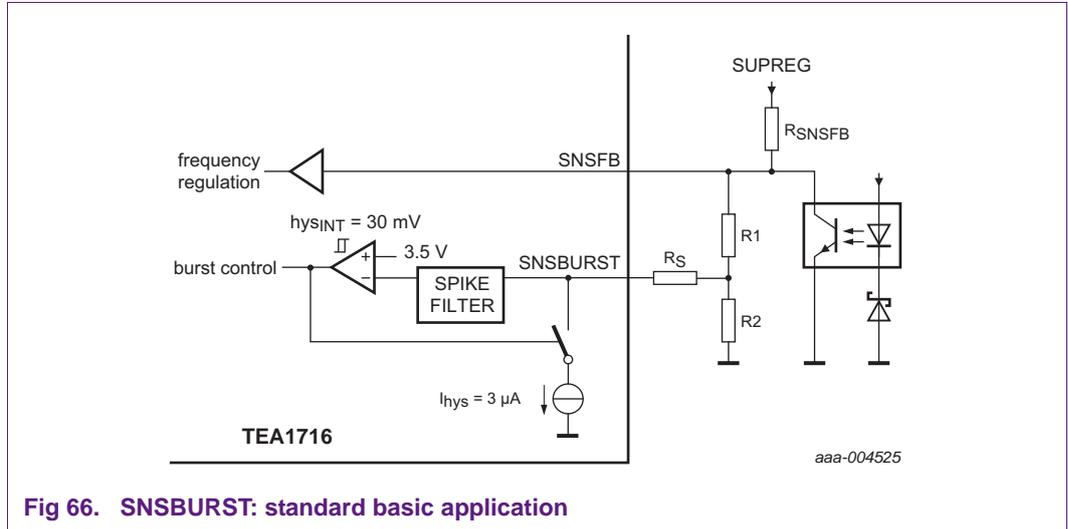
Fig 66. SNSBURST: standard basic application
