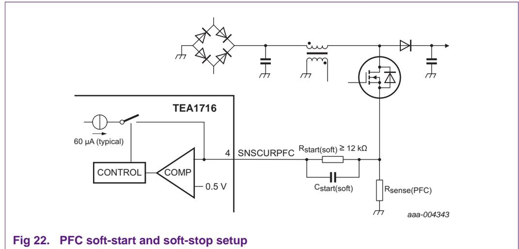
**Fig 22. PFC soft-start and soft-stop setup**
