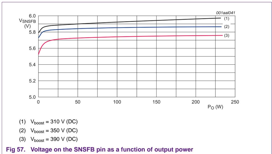
Fig 57. Voltage on the SNSFB pin as a function of output power
