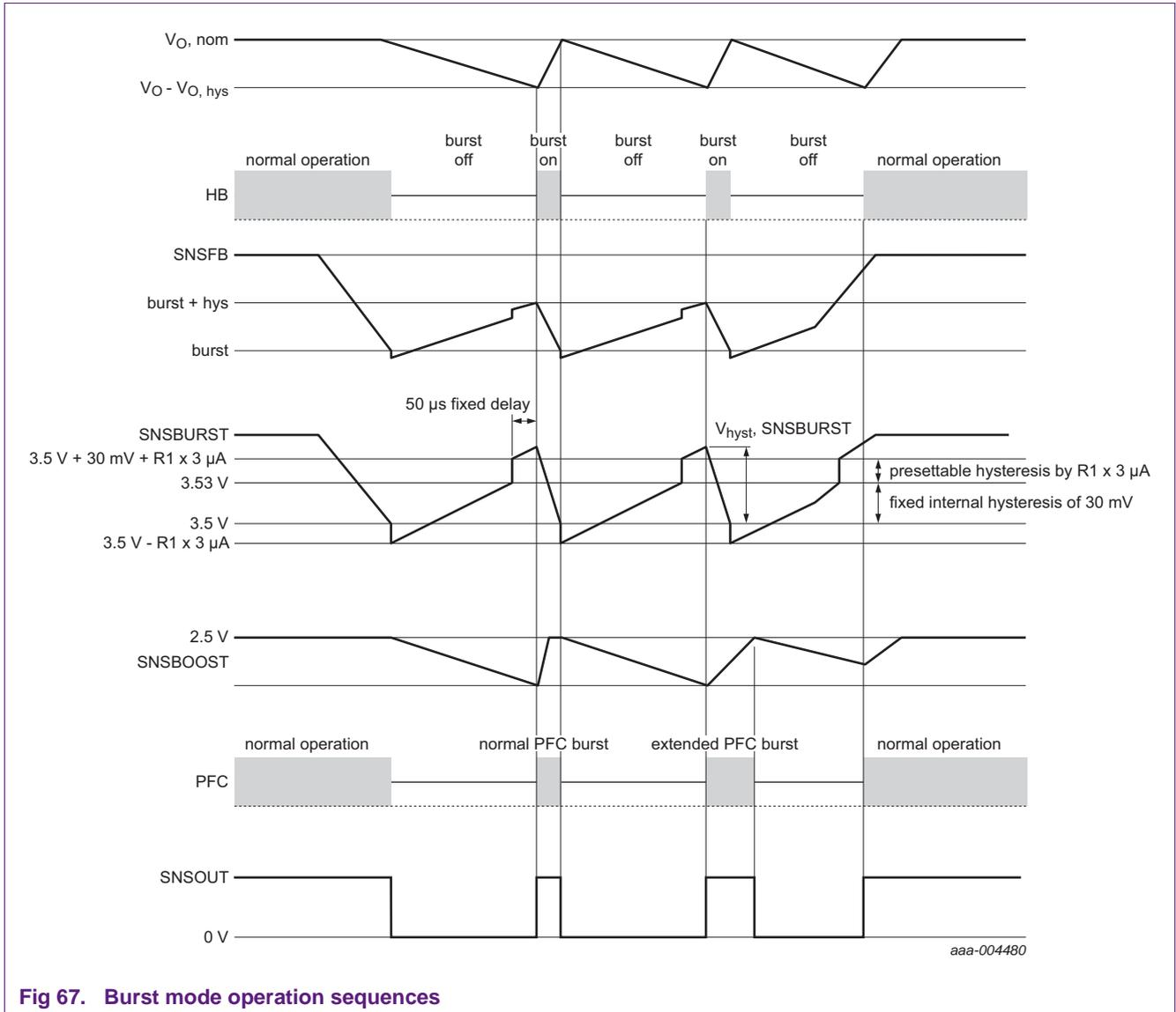
Fig 67. Burst mode operation sequences
