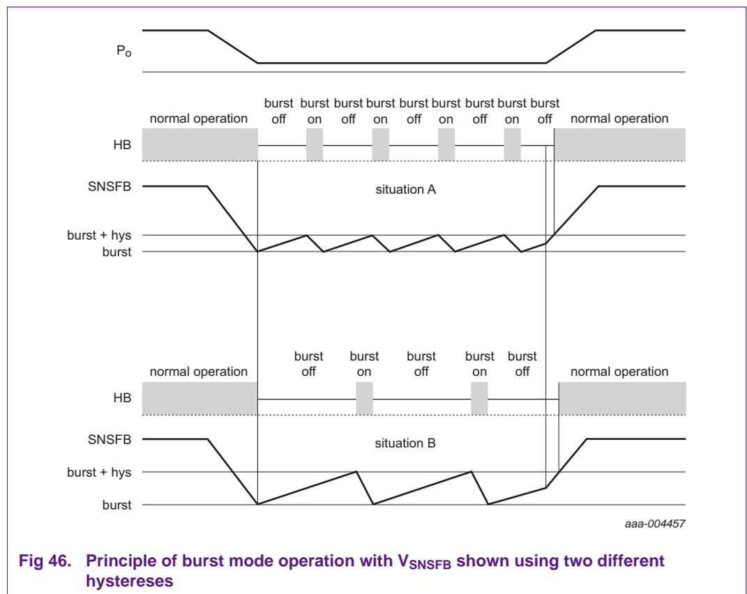
Fig 46. Principle of burst mode operation with  $V_{SNSFB}$  shown using two different hystereses
