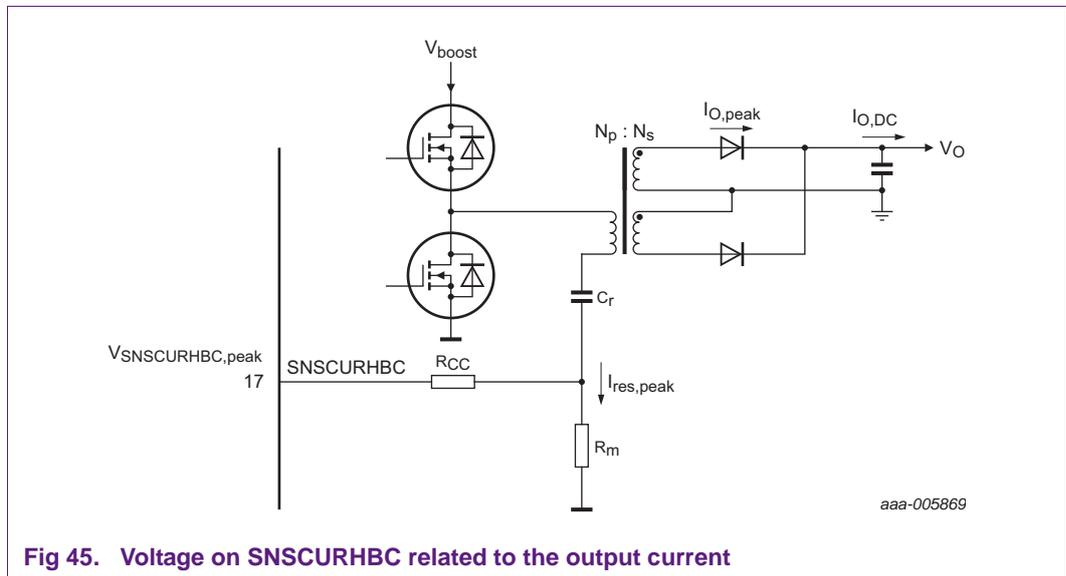
The relationship between the voltage on the SNSCURHBC pin and the primary converter current is defined by measuring resistor  $R_m$ .
