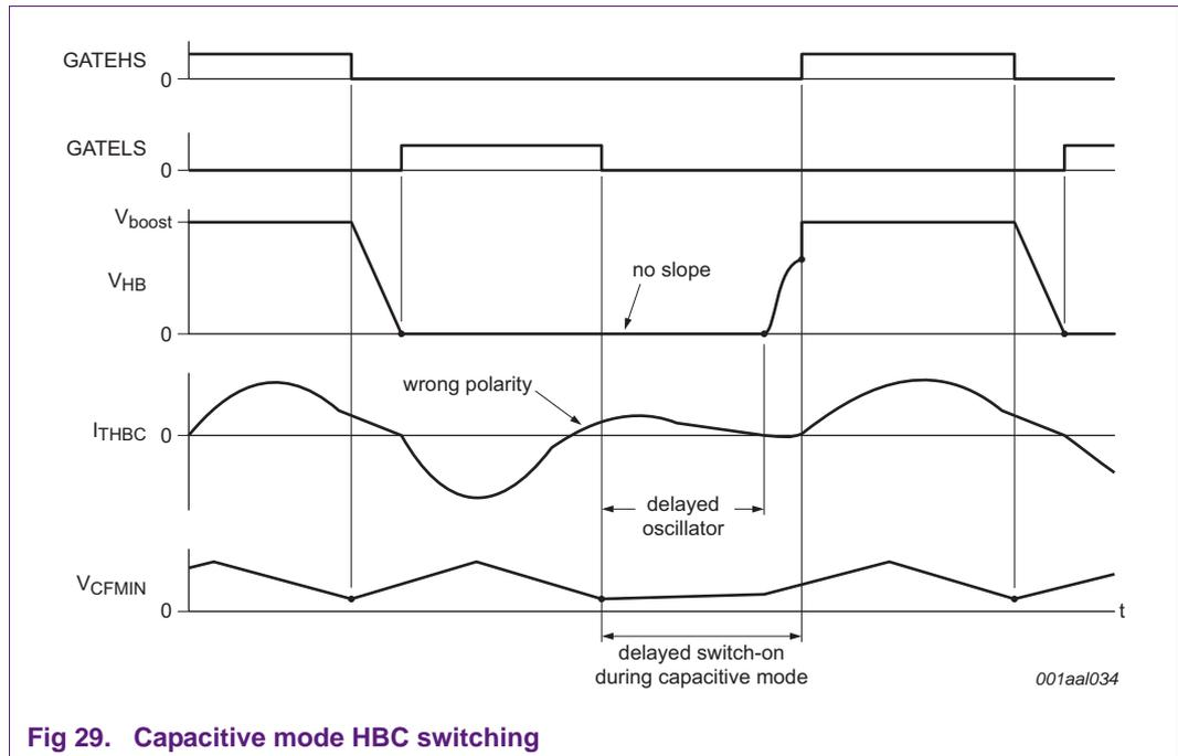
Fig 29. Capacitive mode HBC switching
