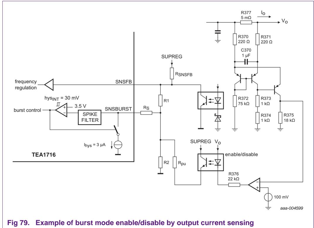
Fig 79. Example of burst mode enable/disable by output current sensing
