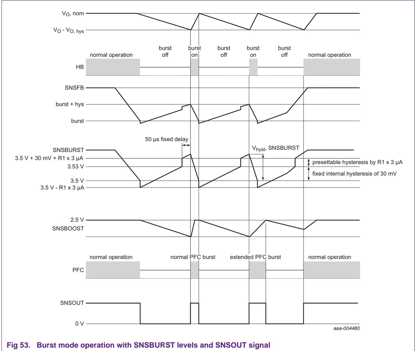
Fig 53. Burst mode operation with SNSBURST levels and SNSOUT signal
