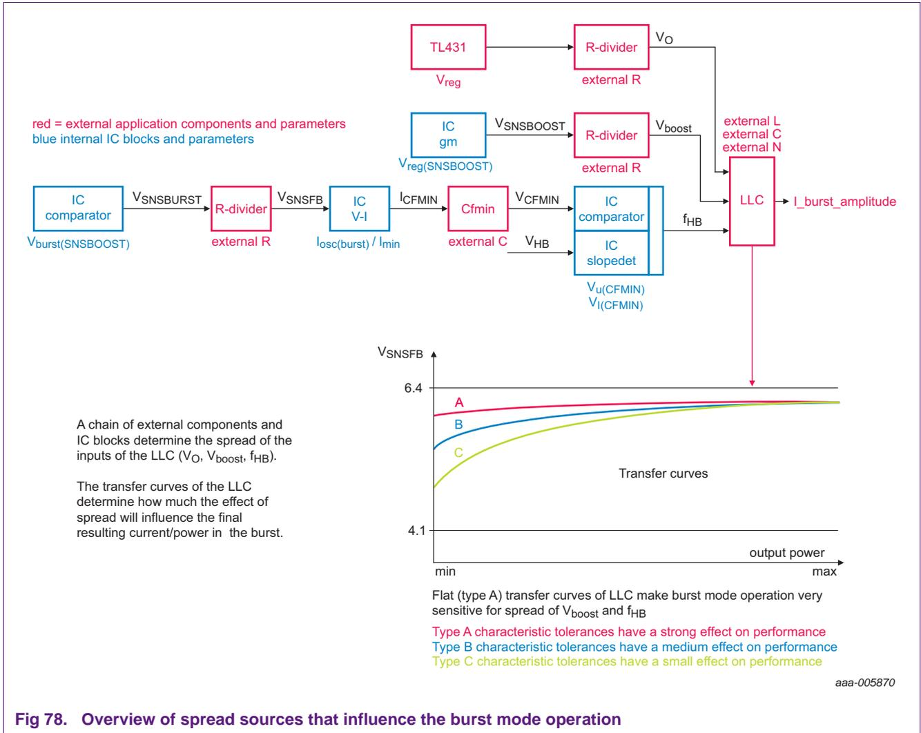
Fig 78. Overview of spread sources that influence the burst mode operation
