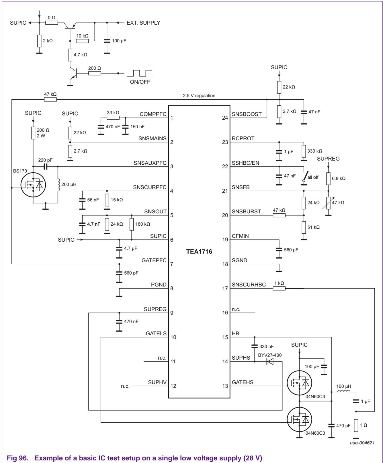
Fig 96. Example of a basic IC test setup on a single low voltage supply (28 V)
