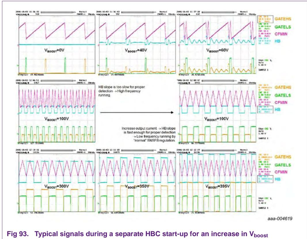
Fig 93. Typical signals during a separate HBC start-up for an increase in  $V_{boost}$
