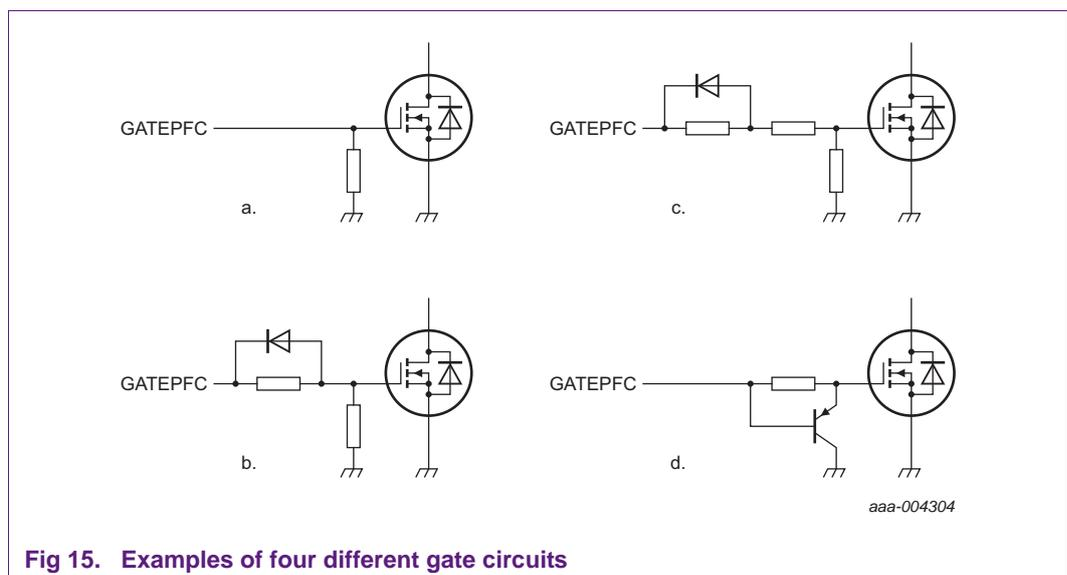
Fig 15. Examples of four different gate circuits
