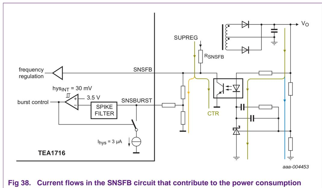
Fig 38. Current flows in the SNSFB circuit that contribute to the power consumption
