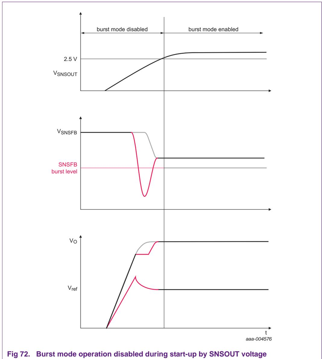
When the SNSOUT pin reaches 2.5 V, burst mode operation is enabled and remains enabled until the TEA1716 stops operating and restarts, a restart or start-up is made.
