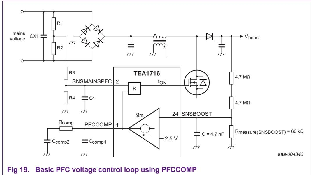
Fig 19. Basic PFC voltage control loop using PFCCOMP
