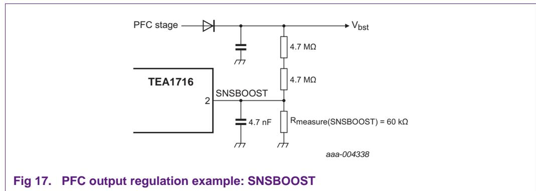
The boost output voltage value is set between the PFC output voltage and the SNSBOOST pin using a resistor divider. When in regulation, the SNSBOOST voltage is kept at 2.5 V.
