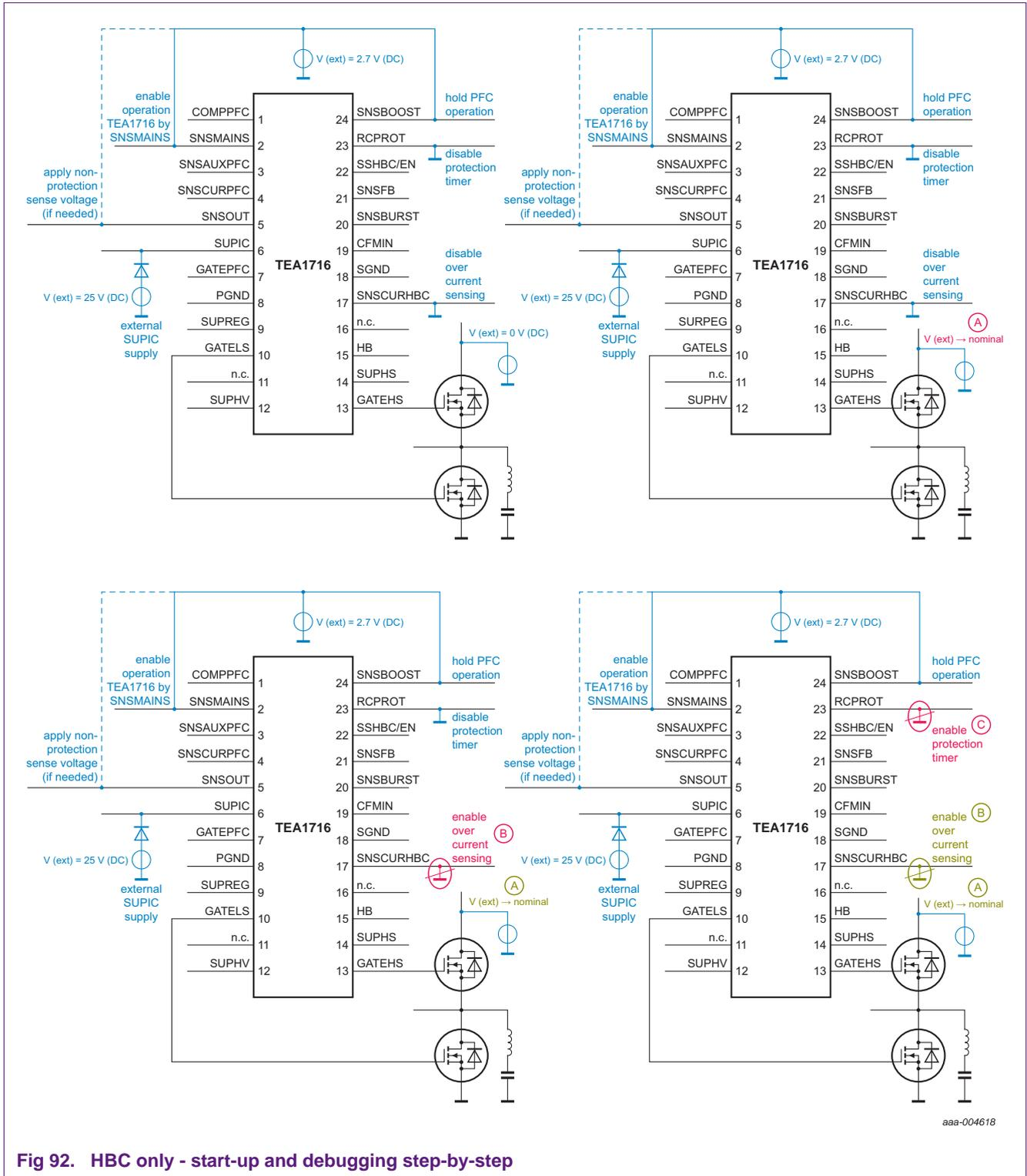
Fig 92. HBC only - start-up and debugging step-by-step
