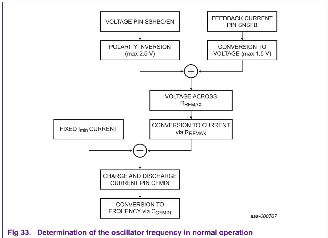
Fig 33. Determination of the oscillator frequency in normal operation
