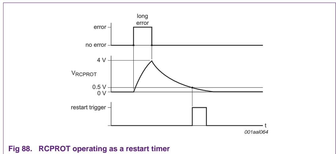
Fig 88. RCPROT operating as a restart timer
