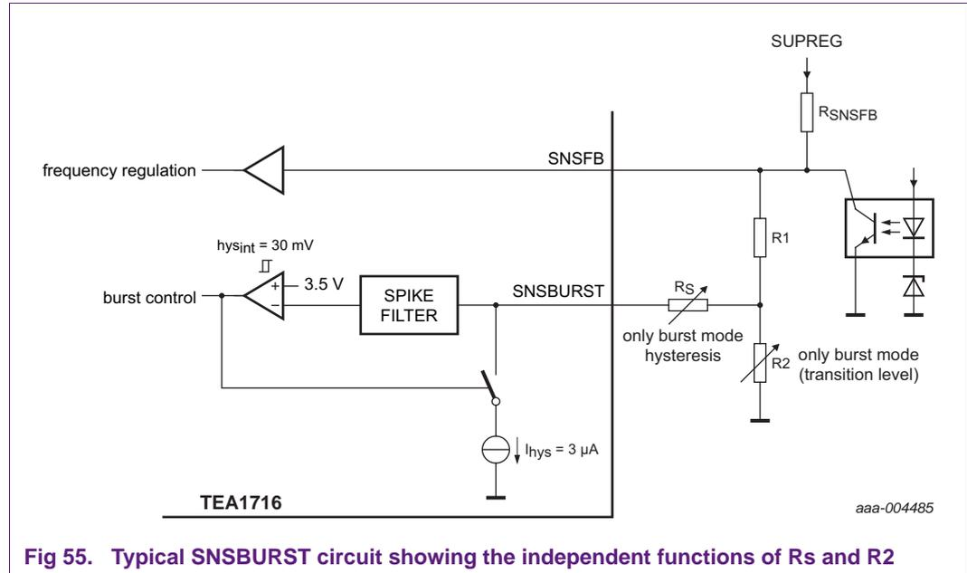
Fig 55. Typical SNSBURST circuit showing the independent functions of  $R_S$  and  $R_2$
