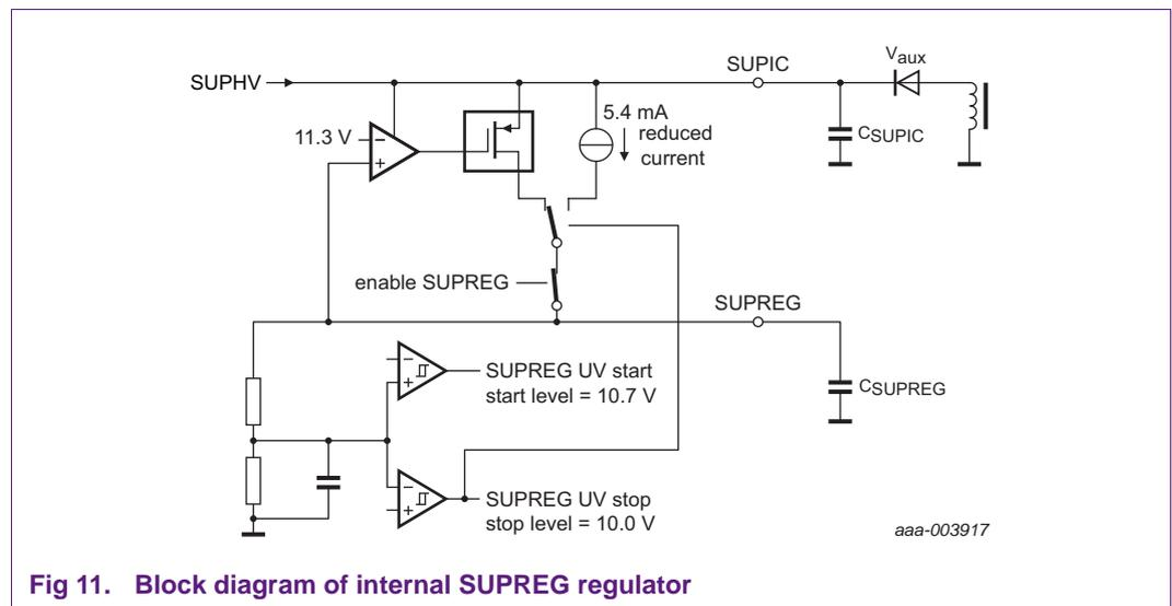
Fig 11. Block diagram of internal SUPREG regulator
