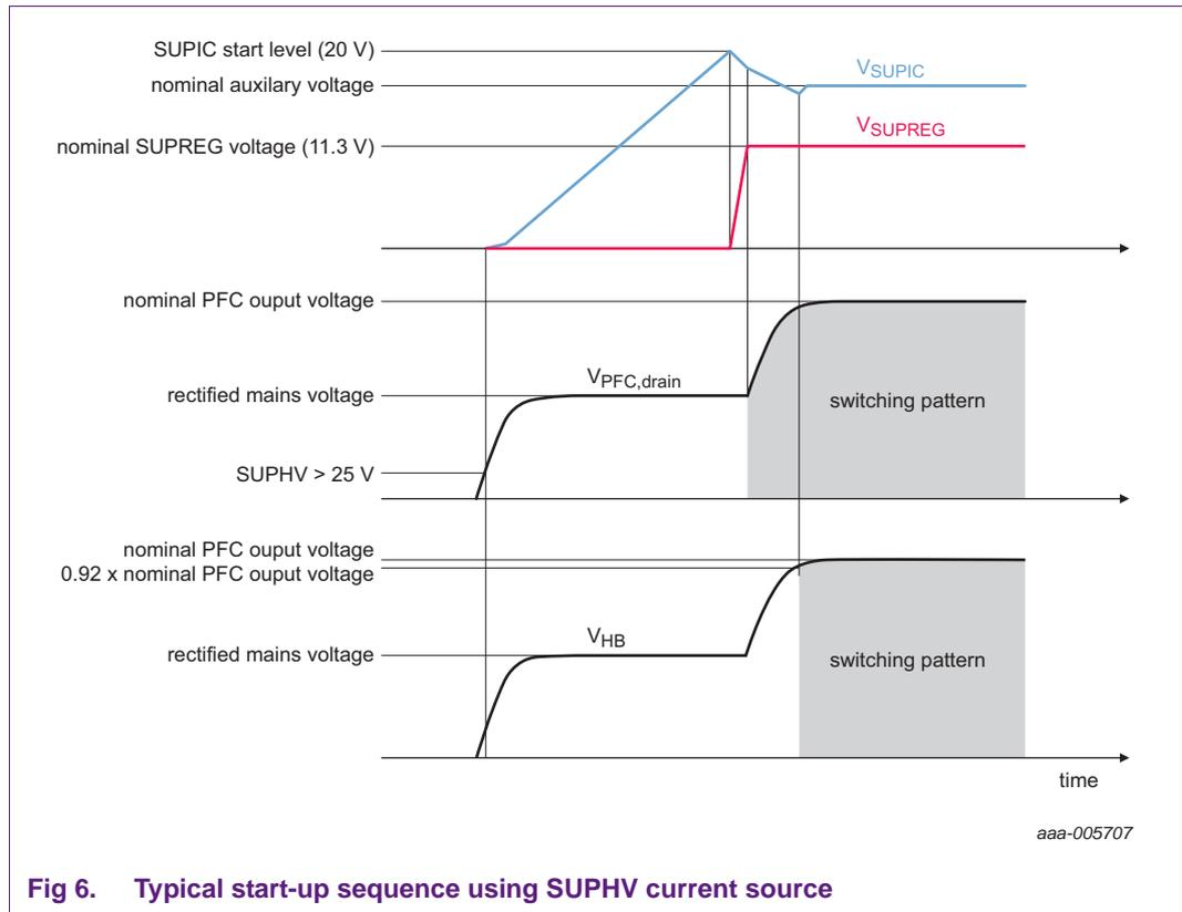
Fig 6. Typical start-up sequence using SUPHV current source
