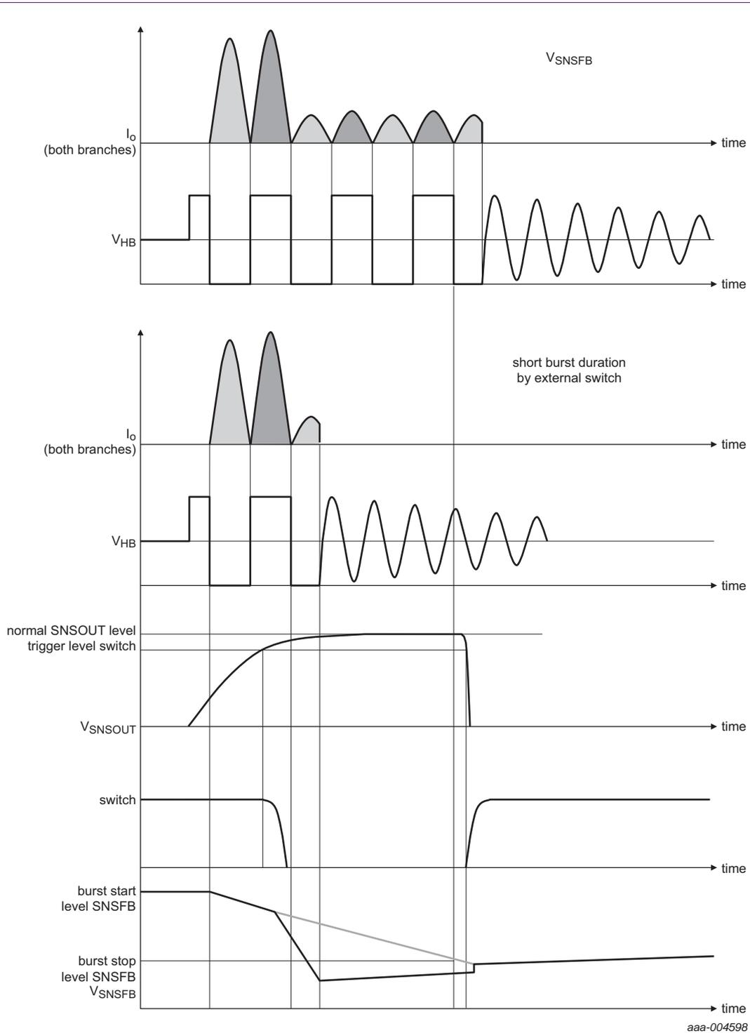
Fig 77. Shorter burst duration by external switch
