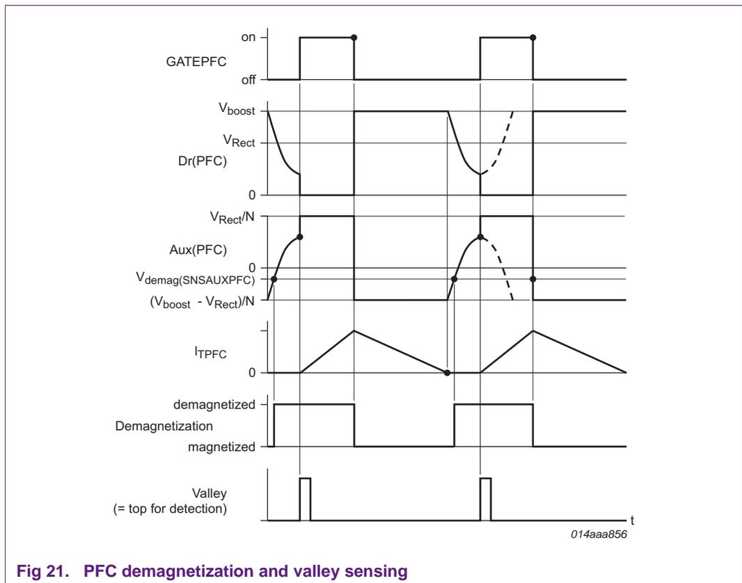
Fig 21. PFC demagnetization and valley sensing
