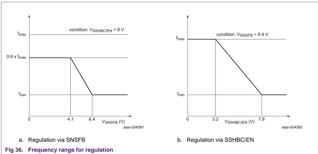
**Fig 36. Frequency range for regulation**
