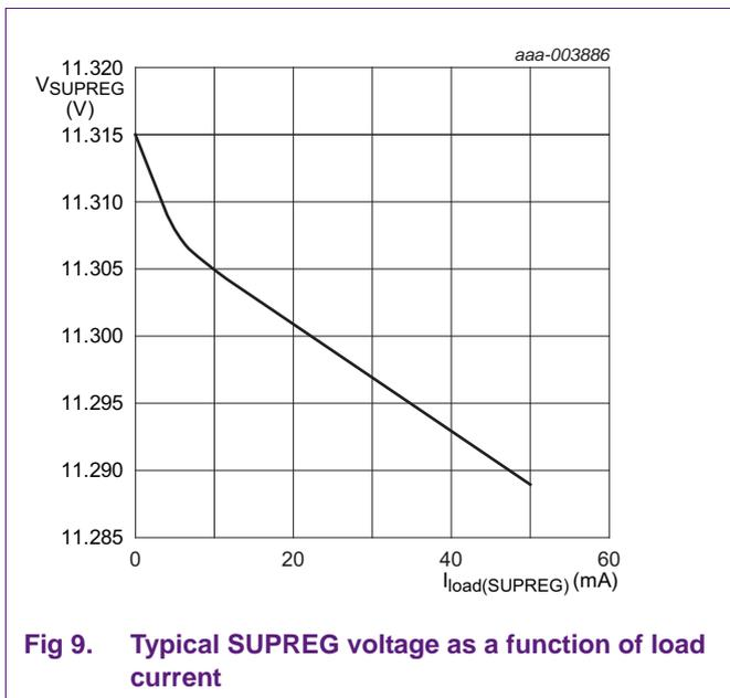
Fig 9. Typical SUPREG voltage as a function of load current
