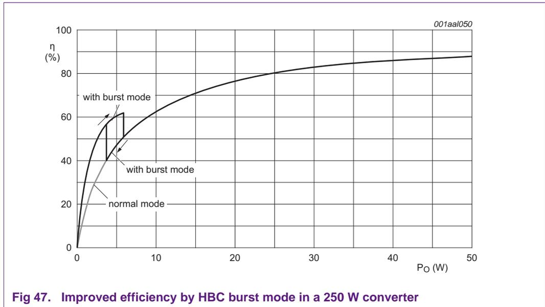
Fig 47. Improved efficiency by HBC burst mode in a 250 W converter
