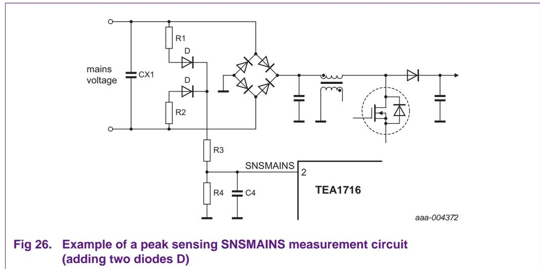
Fig 26. Example of a peak sensing SNSMAINS measurement circuit (adding two diodes D)
