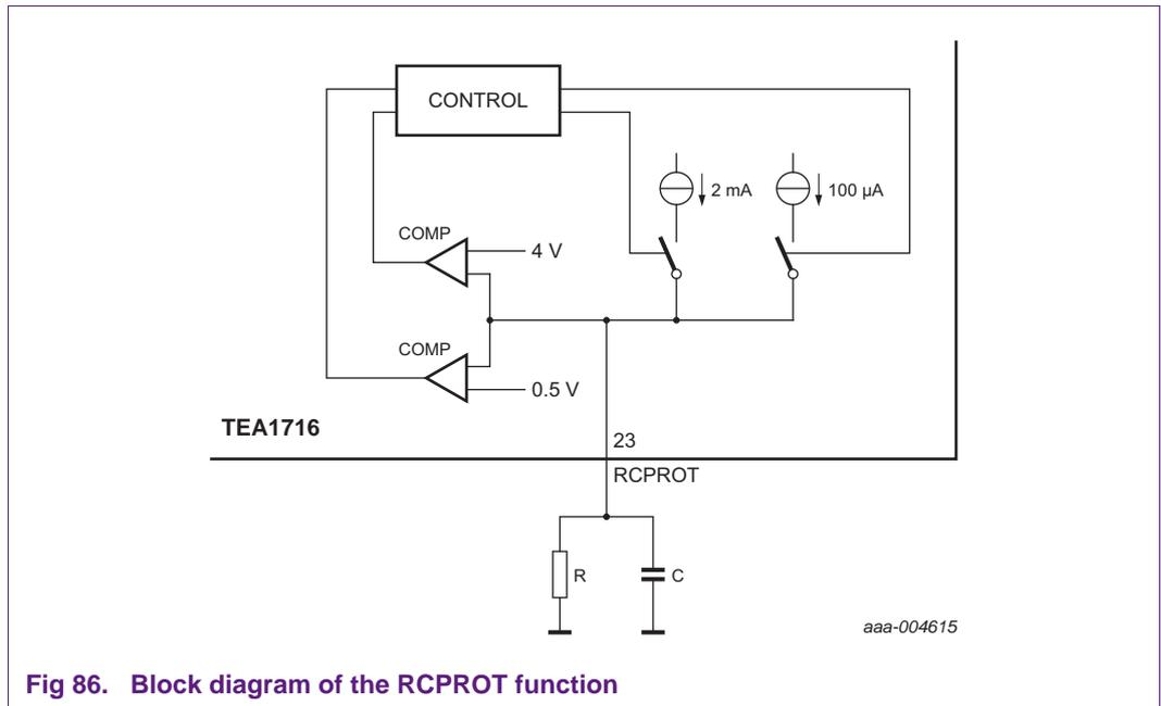
Fig 86. Block diagram of the RCPROT function
