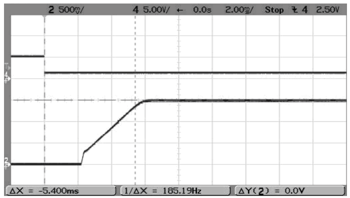
On/Off Enable Startup (V in =5V, V out =1.5V, I out =6A, Cload=0) Trace 4=Enable, Trace2=Vout
