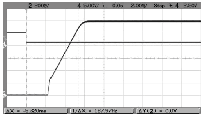
On/Off Enable Startup (V in =5V, V out =1.2V, I out =6A, Cload=0) Trace 4=Enable, Trace 2=Vout
