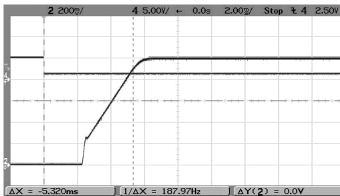
On/Off Enable Startup (V IN =5V, V OUT =1.0V, I OUT =6A, C LOAD =0) Trace 4=Enable, Trace 2=V OUT
