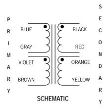
$<sup>^{\</sup>mathrm{1}}$  Primary and secondary windings are designed to be connected in series or parallel. Windings are not intended to be used independently.
