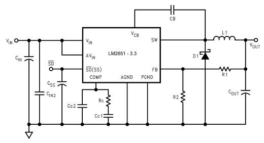
Figure 1. LM2651\_EVAL Schematic for Adjustable Voltage
