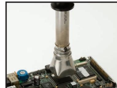
Efficiently desolders QFPs and other SMT components
