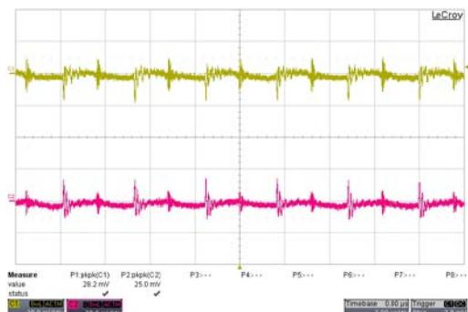
Typical Output Ripple and Noise.
