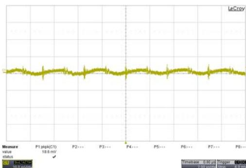
Typical Output Ripple and Noise.
