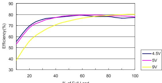
Efficiency Versus Output Current
