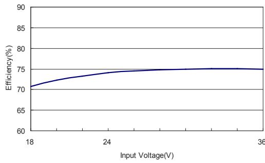
Efficiency Versus Input Voltage. Full Load
