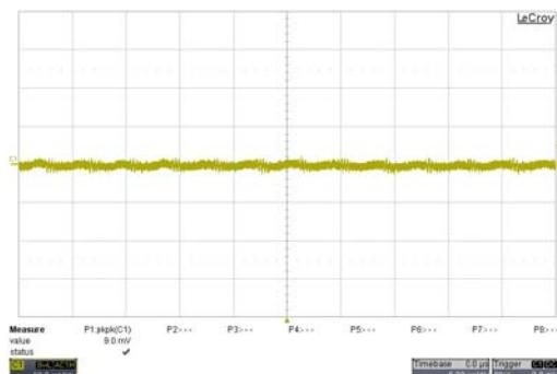
Typical Output Ripple and Noise.
