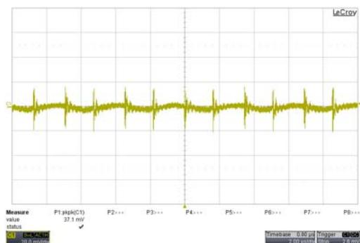
Typical Output Ripple and Noise.
