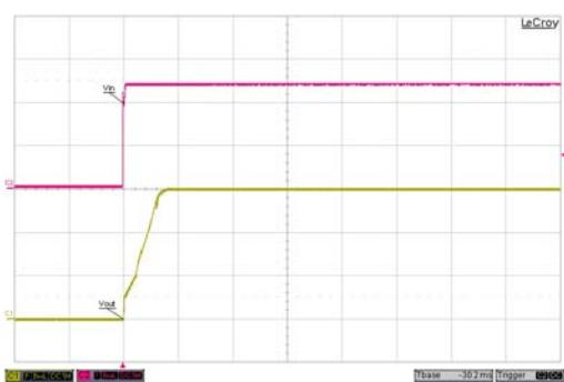
Typical Input Start-Up and Output Rise Characteristic
