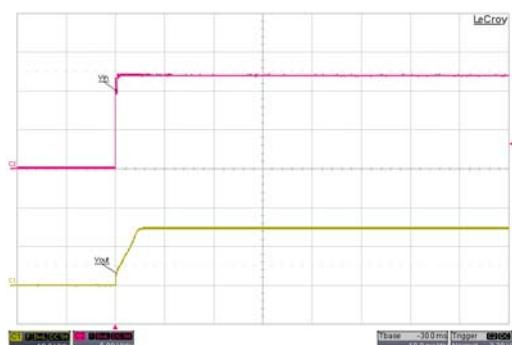
Typical Input Start-Up and Output Rise Characteristic
