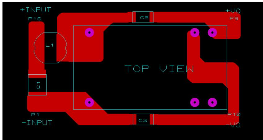
Recommended PCB Layout with Input Filter
