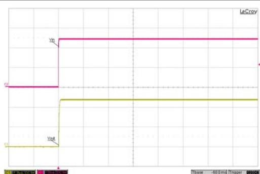
Typical Input Start-Up and Output Rise Characteristic
