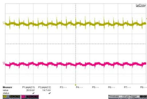
Typical Output Ripple and Noise.
