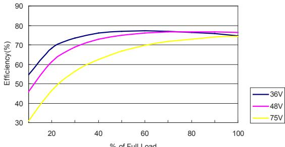
Efficiency Versus Output Current
