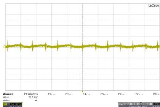
Typical Output Ripple and Noise.
