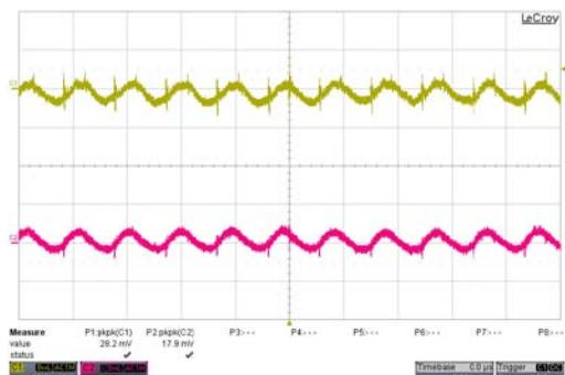
Typical Output Ripple and Noise.
