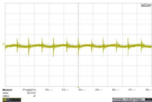
Typical Output Ripple and Noise.
