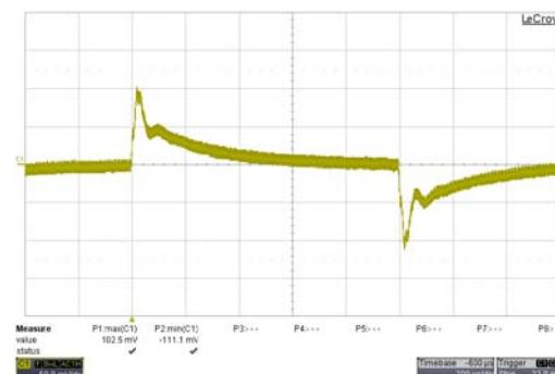
Transient Response to Dynamic Load Change from 100% to 75% of Full Load ;  $V_{in} = V_{in \text{ nom}}$
