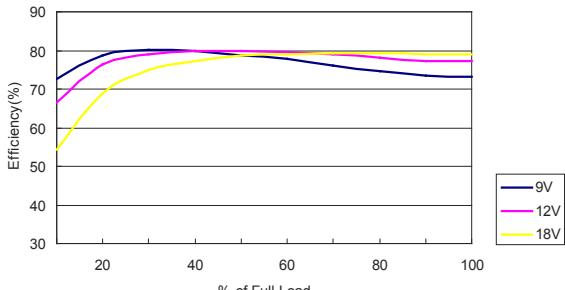
Efficiency Versus Output Current
