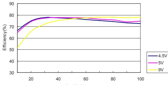
Efficiency Versus Output Current
