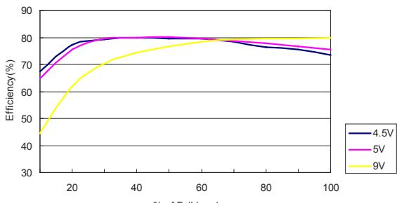
Efficiency Versus Output Current
