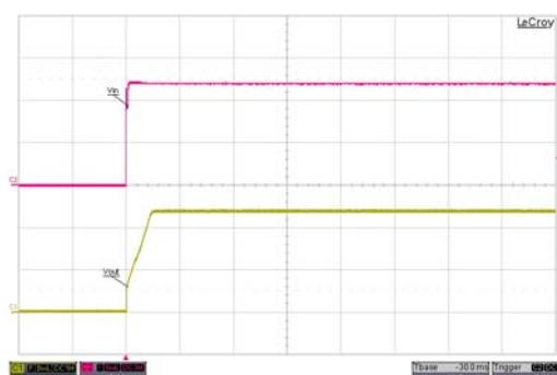
Typical Input Start-Up and Output Rise Characteristic
