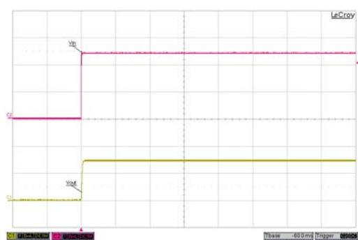
Typical Input Start-Up and Output Rise Characteristic
