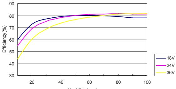
Efficiency Versus Output Current
