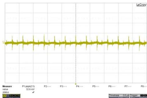
Typical Output Ripple and Noise.
