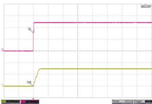
Typical Input Start-Up and Output Rise Characteristic
