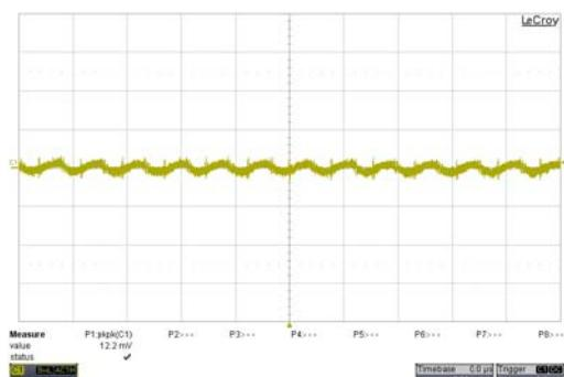
Typical Output Ripple and Noise.
