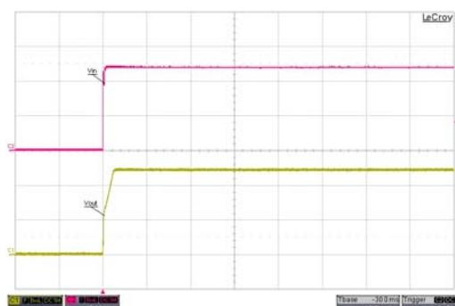
Typical Input Start-Up and Output Rise Characteristic
