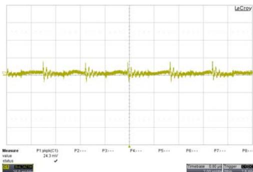
Typical Output Ripple and Noise.
