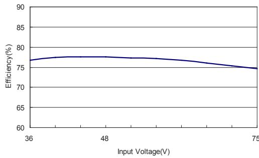
Efficiency Versus Input Voltage. Full Load
