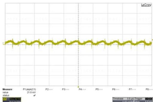
Typical Output Ripple and Noise.
