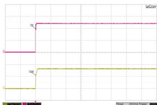
Typical Input Start-Up and Output Rise Characteristic
