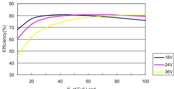
Efficiency Versus Output Current
