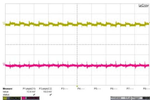
Typical Output Ripple and Noise.
