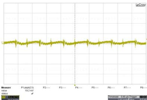
Typical Output Ripple and Noise.
