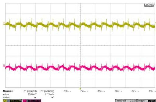
Typical Output Ripple and Noise.
