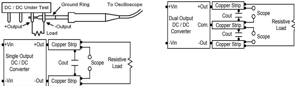
**Output voltage and efficiency measurement test up**
