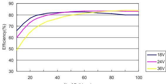
Efficiency Versus Output Current
