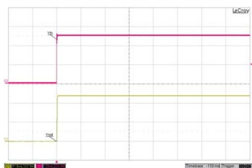
Typical Input Start-Up and Output Rise Characteristic
