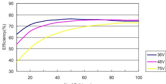
Efficiency Versus Output Current
