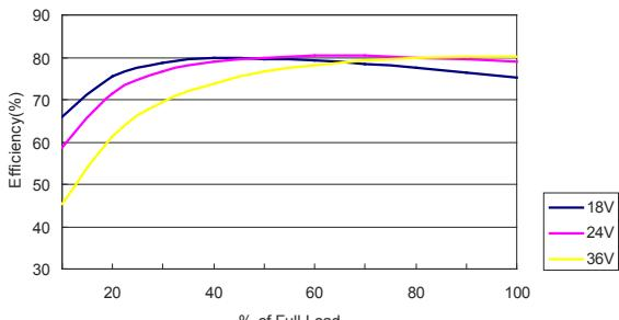
Efficiency Versus Output Current
