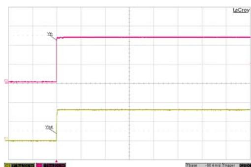
Typical Input Start-Up and Output Rise Characteristic
