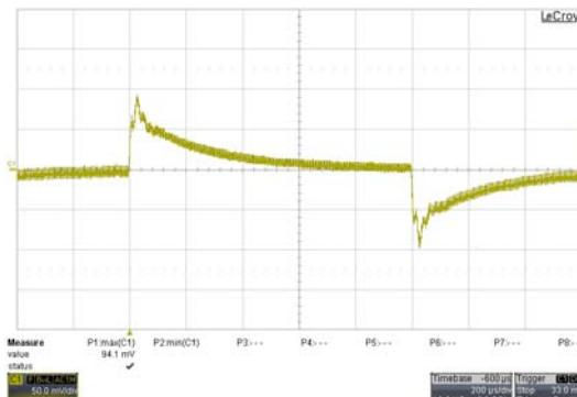
Transient Response to Dynamic Load Change from 100% to 75% of Full Load ;  $V_{in} = V_{in \text{ nom}}$
