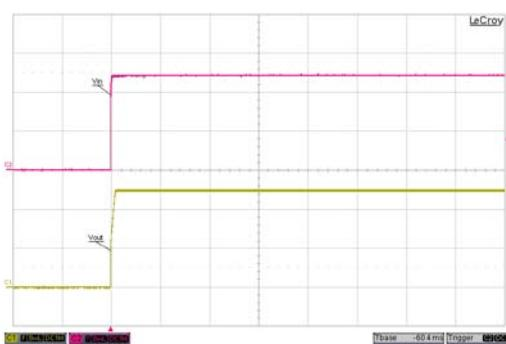
Typical Input Start-Up and Output Rise Characteristic
