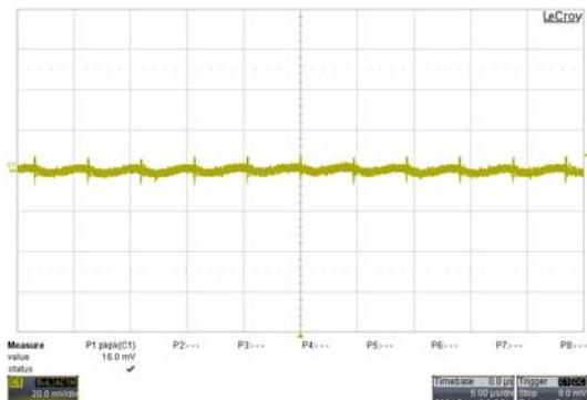
Typical Output Ripple and Noise.
