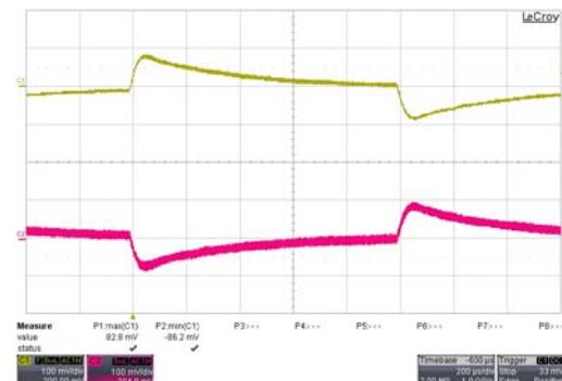
Transient Response to Dynamic Load Change from 100% to 75% of Full Load ;  $V_{in} = V_{in\ nom}$
