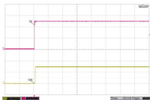
Typical Input Start-Up and Output Rise Characteristic
