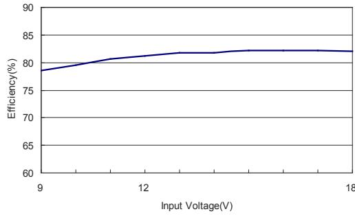
Efficiency Versus Input Voltage. Full Load
