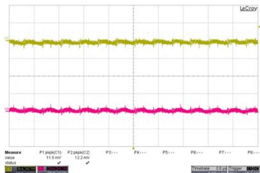
Typical Output Ripple and Noise.
