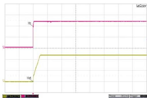
Typical Input Start-Up and Output Rise Characteristic
