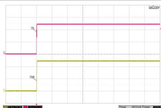
Typical Input Start-Up and Output Rise Characteristic
