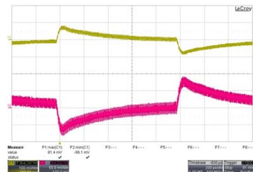
Transient Response to Dynamic Load Change from 100% to 75% of Full Load ;  $V_{in} = V_{in\ nom}$
