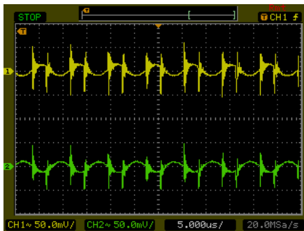
Typical Output Ripple and Noise. V_{in} = V_{in\ nom} ; Full Load; T_A = +25^\circ C
