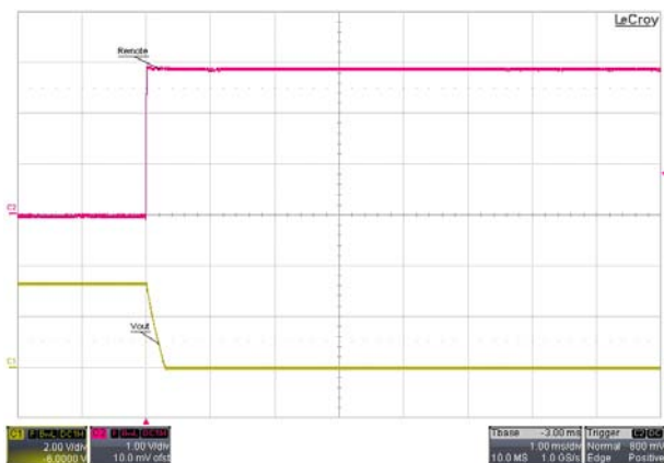
Using ON/OFF Voltage Start-Up and V_{out} Rise Characteristic V_{in} = V_{in\ nom} ; Full Load
