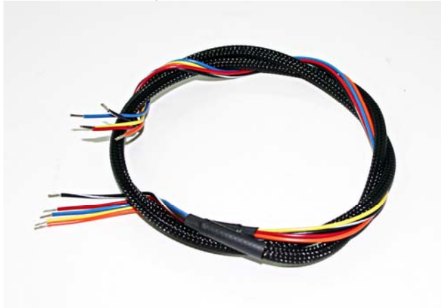
Figure 2: 5-wire cable for step, direction, disable, 5V output & opto supply
