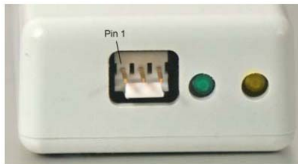
RS485 Connection View
