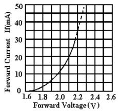
Forward current vs. Forward Voltage
