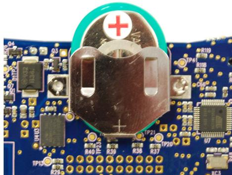
If the battery is connected while the USB power source is being used, a trickle charge of the battery occurs.
