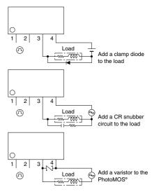
2) Even if spike voltages generated at the load are limited with a clamp diode or snubber circuit if the circuit wires are long, spike voltages will occur by inductance. Keep wires as short as possible to minimize inductance.
