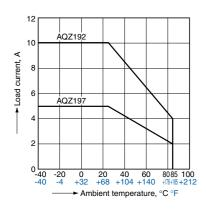
2. Load current vs. ambient temperature characteristics in adjacent mounting Sample: All types
