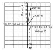
10. Leakage current vs. load voltage characteristics
