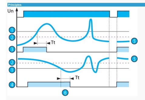
If "with memory" mode has been selected, the relay opens and stays in this position when threshold crossing is detected. The power supply must be disconnected to reset the product.
