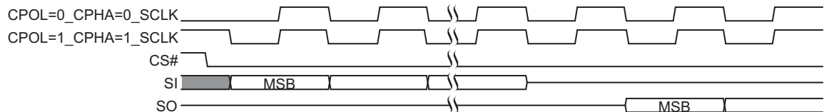
Figure 4.1 SPI Modes Supported
