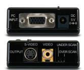
The SY-PT385A is a PC to Video scan converter which is designed to convert a variety of PC analogue video signals from VGA to WUXGA. This device also converts between interlaced NTSC or PAL video and features a frame rate conversion function in addition to an Overscan / Underscan function that allows users to view a PC source on a Composite or S-Video monitor without cropping the images.
