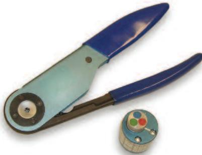
This is a ratcheted, four indent crimptool that is fully adjustable. They crimp all sizes of machined and coaxial contacts.
