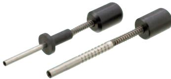
Contacts can readily be removed from the housings using an extraction tool. The tool is placed over the contact and the sleeve rotated slightly as it is pushed home to release the spring. Light pressure on the knob then ejects the contact from the rear of the housing.
