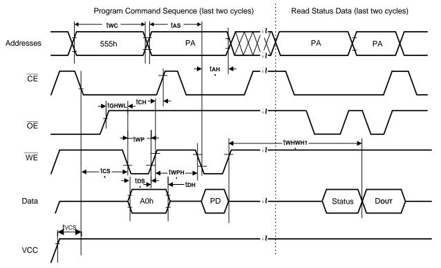
Note : PA = program addrss, PD = program data, Dout is the true data at the program address.
