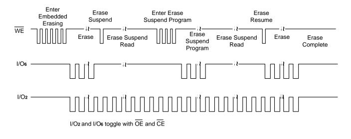
Note : Both I/O<sub>6</sub> and I/O<sub>2</sub> toggle with OE or CE. See the text on I/O<sub>6</sub> and I/O<sub>2</sub> in the section "Write Operation Statue" for more information.
