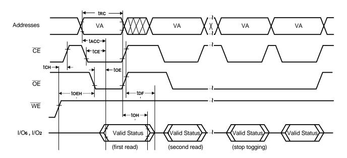
Note: VA = Valid Address; not required for I/O<sub>6</sub>. Illustration shows first two status cycle after command sequence, last status read cycle, and array data read cycle.
