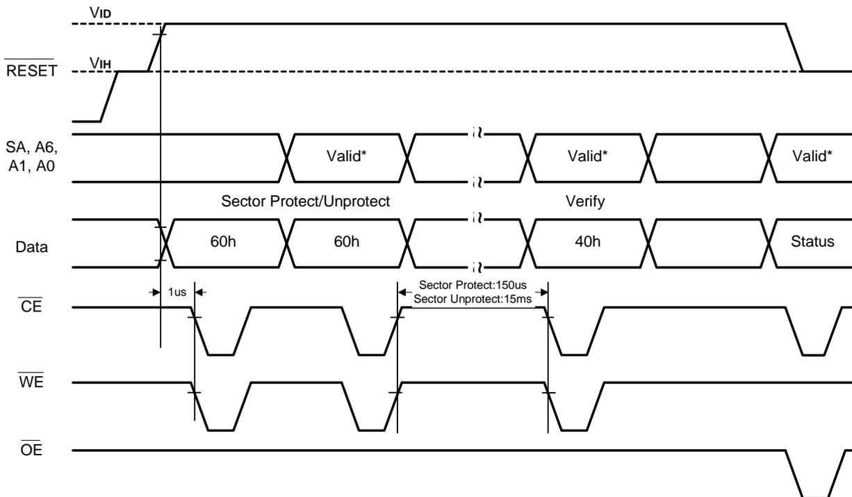
Note : For sector protect, A<sub>6</sub>=0, A<sub>1</sub>=1, A<sub>0</sub>=0. For sector unprotect, A<sub>6</sub>=1, A<sub>1</sub>=1, A<sub>0</sub>=0
