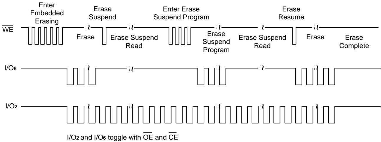
Note : Both I/O<sub>6</sub> and I/O<sub>2</sub> toggle with  $\overline{OE}$  or  $\overline{CE}$ . See the text on I/O<sub>6</sub> and I/O<sub>2</sub> in the section "Write Operation Status" for more information.
