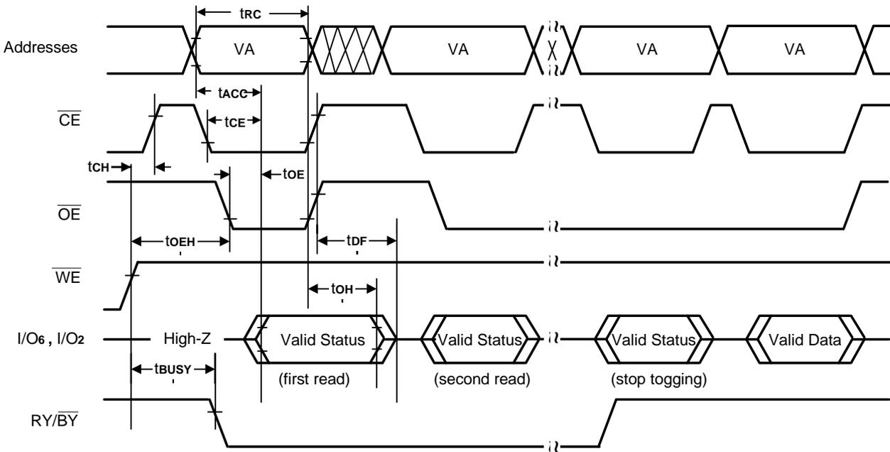
Note: VA = Valid Address; not required for I/O<sub>6</sub>. Illustration shows first two status cycle after command sequence, last status read cycle, and array data read cycle.
