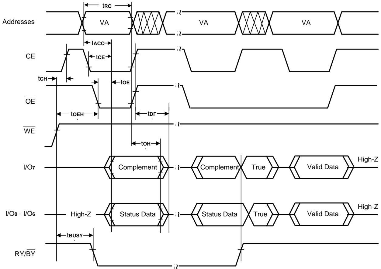
Note : VA = Valid Address. Illustration shows first status cycle after command sequence, last status read cycle, and array data read cycle.
