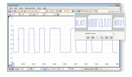
To help you find you way around the buffer memory, you can divide it into as many as 10,000 individually triggered segments. Use the visual buffer navigator to scan through the segments, or set up a mask to filter out the waveforms of interest.
