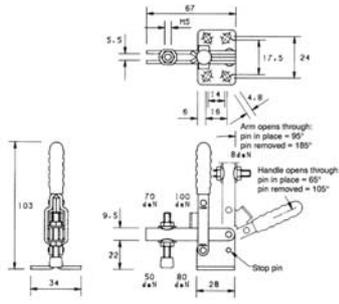
Adjustable spindle positioning along the arm with straight base. 100daN holding force. Supplied with set screw, nuts, neoprene cover and flanged washers.
