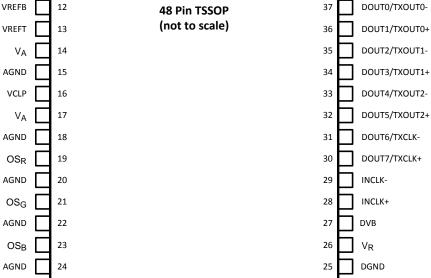
Figure 2. LM98714 Pin Out Diagram
