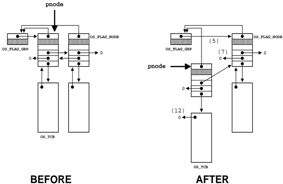
**Figure 9.8** *Removing an OS\_FLAG\_NODE from the wait list, Case C.*
