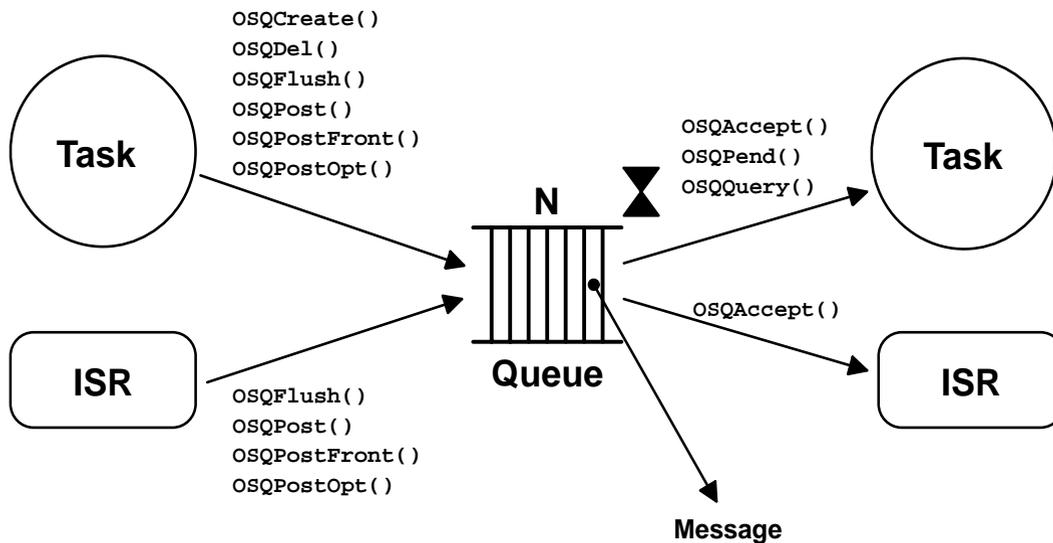
**Figure 11.2** *Data structures used in a message queue.*
