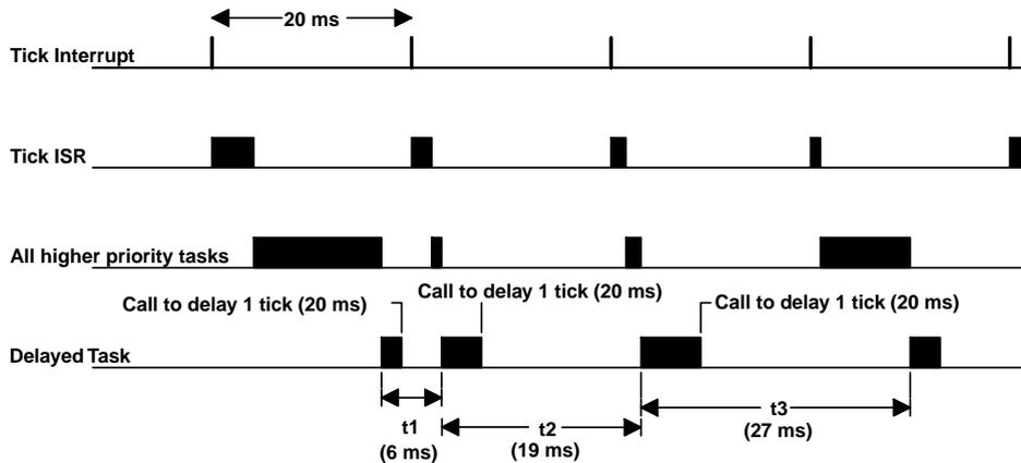
Case 3 (Figure 2.27) shows a situation in which the execution times of all higher priority tasks and ISRs extend beyond one clock tick. In this case, the task that tries to delay for one tick actually executes two ticks later and misses its deadline. Missing the deadline might be acceptable in some applications, but in most cases it isn't.
