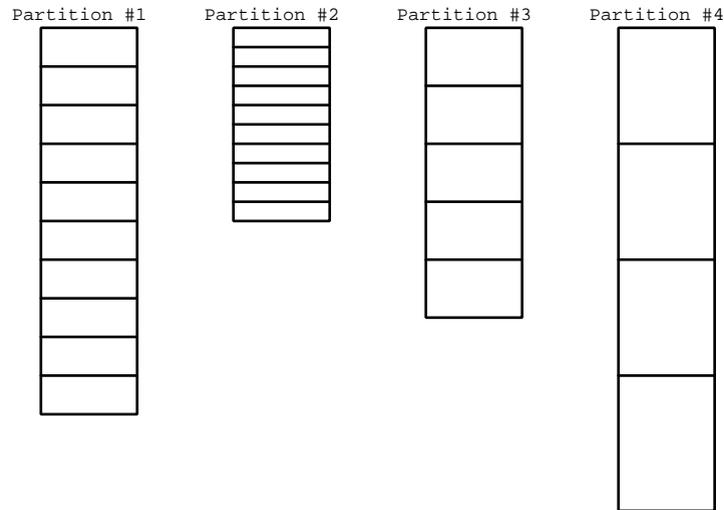
$\mu\text{C}/\text{OS-II}$  initializes the memory manager if you configure `OS_MEM_EN` to 1 in `OS_CFG.H`. Initialization is done by `OS_MemInit()` [called by `OSInit()`] and consists of creating a linked list of memory control blocks, as shown in Figure 12.3. You specify the maximum number of memory partitions with the configuration constant `OS_MAX_MEM_PART` (see `OS_CFG.H`), which must be set at least to 2.
