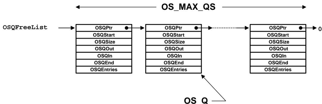
A *queue control block* is a data structure used to maintain information about the queue. It contains the fields described in the following list. Note that the fields are preceded with a dot to show that they are members of a structure, as opposed to simple variables.
