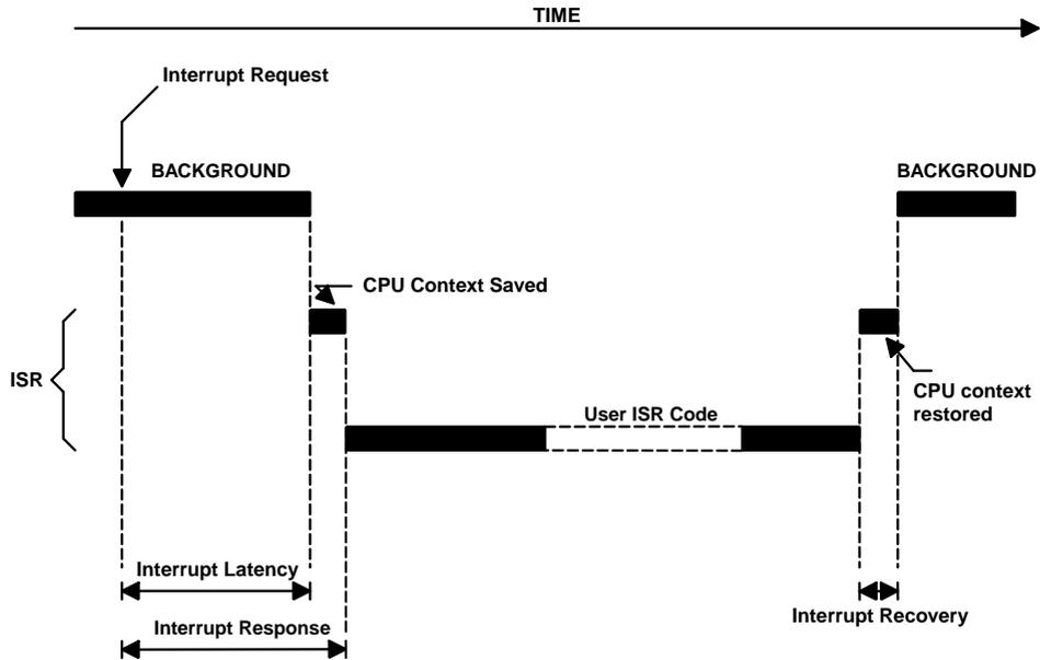
**Figure 2.21** *Interrupt latency, response, and recovery (non-preemptive kernel).*
