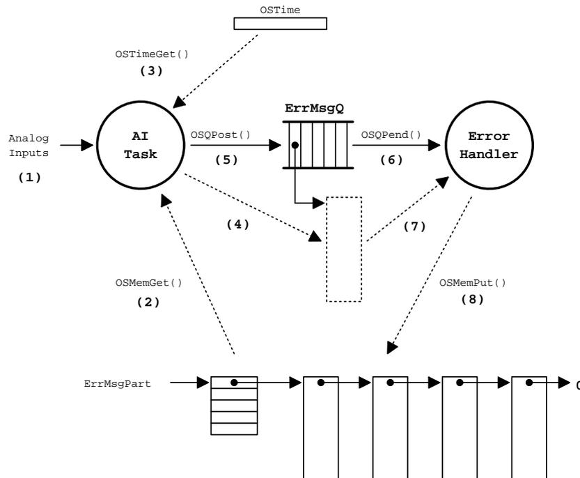
The first task reads and checks the value of analog inputs (pressures, temperatures, and voltages) and sends a message to the second task if any of the analog inputs exceed a threshold. The message sent contains a time stamp, information about which channel had the error, an error code, an indication of the severity of the error, and any other information you can think of.
