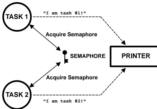
The above example implies that each task must know about the existence of the semaphore in order to access the resource. In some situations, it is better to encapsulate the semaphore. Each task would thus not know that it is actually acquiring a semaphore when accessing the resource. For example, an RS-232C port is used by multiple tasks to send commands and receive responses from a device connected at the other end (Figure 2.11).
