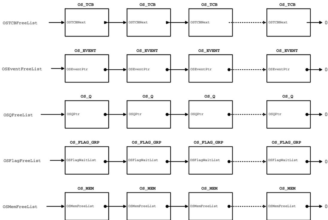
After OSInit() has been called, the OS\_TCB pool contains OS\_MAX\_TASKS entries. The OS\_EVENT pool contains OS\_MAX\_EVENTS entries, the OS\_Q pool contains OS\_MAX\_QS entries, the OS\_FLAG\_GRP pool contains OS\_MAX\_FLAGS entries, and, finally, the OS\_MEM pool contains OS\_MAX\_MEM\_PART entries. Each of the free pools are NULL-pointer terminated to indicate the end. The pool is, of course, empty if any of the list pointers point to NULL. You define the size of these pools in OS\_CFG.H.
