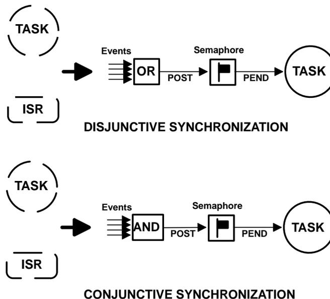
Common events can be used to signal multiple tasks, as shown in Figure 2.16. Events are typically grouped. Depending on the kernel, a group consists of 8, 16, or 32 events, each represented by a bit. (mostly 32 bits, though). Tasks and ISRs can set or clear any event in a group. A task is resumed when all the events it requires are satisfied. The evaluation of which task will be resumed is performed when a new set of events occurs (i.e., during a SET operation).
