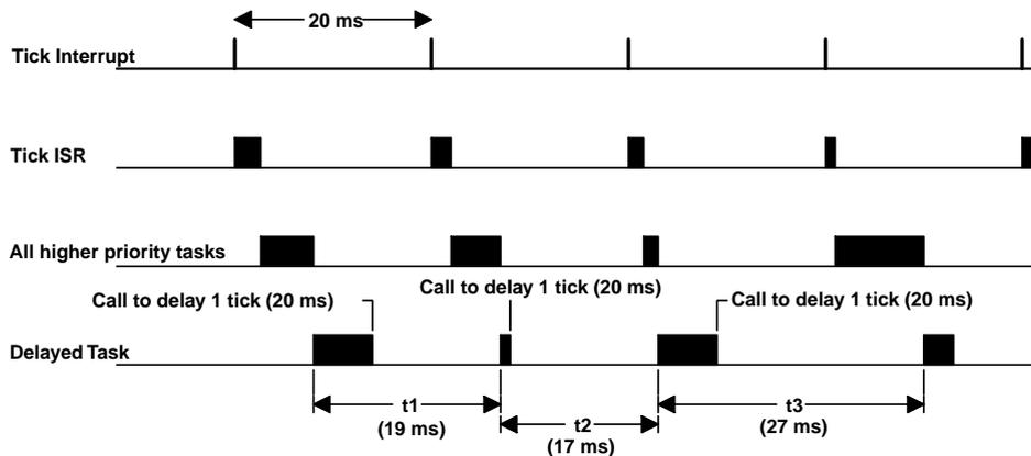
Case 2 (Figure 2.26) shows a situation where the execution times of all higher priority tasks and ISRs are slightly less than one tick. If the task delays itself just before a clock tick, the task executes again almost immediately! Because of this, if you need to delay a task at least one clock tick, you must specify one extra tick. In other words, if you need to delay a task for at least five ticks, you must specify six ticks!
