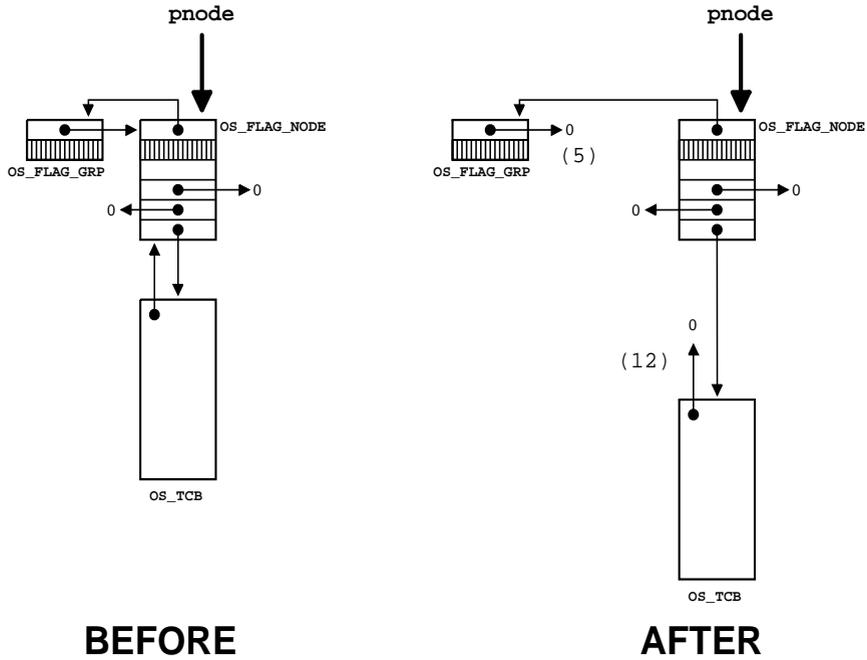
**Figure 9.7** *Removing an OS\_FLAG\_NODE from the wait list, Case B.*
