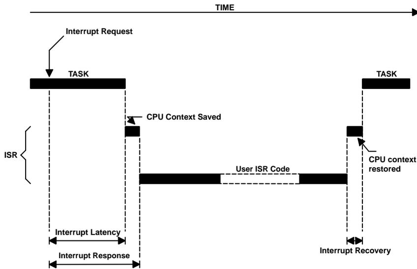
**Figure 2.22** *Interrupt latency, response, and recovery (preemptive kernel).*
