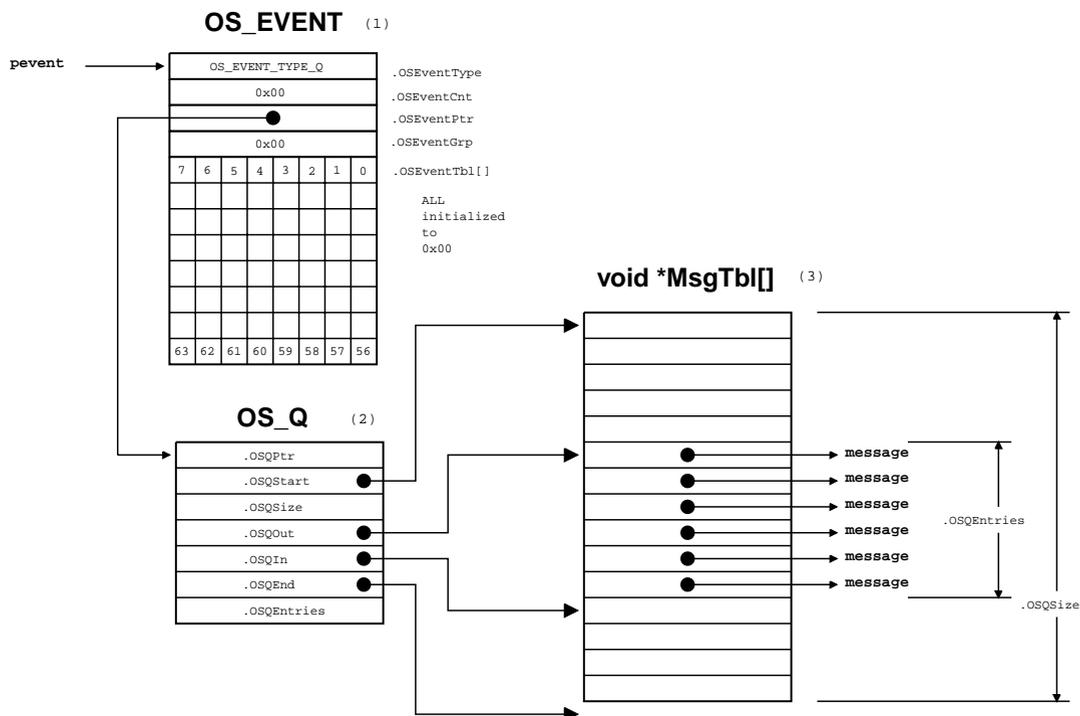
Figure 11.2 shows the different data structures needed to implement a message queue.
