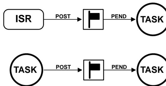
If the kernel supports counting semaphores, the semaphore accumulates events that have not yet been processed. Note that more than one task can be waiting for an event to occur. In this case, the kernel signals the occurrence of the event either to
