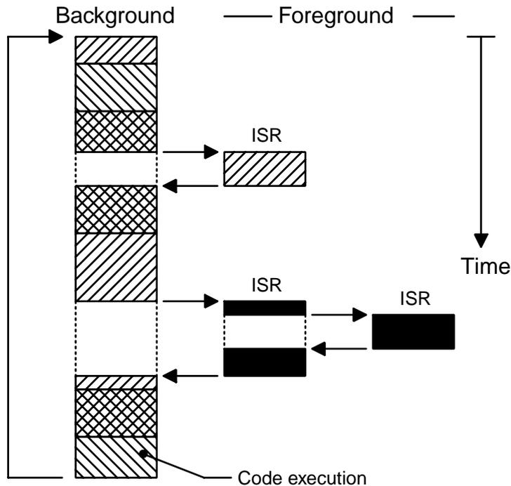
Most high-volume microcontroller-based applications (e.g., microwave ovens, telephones, toys, and so on) are designed as foreground/background systems. Also, in microcontroller-based applications, it might be better (from a power consumption point of view) to halt the processor and perform all of the processing in ISRs.
