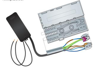
6 When fitting the cables into the cable clamp the sides of the box need to be eased apart to make an opening. It is normal for the entrance to be splayed apart with the cables in place.
