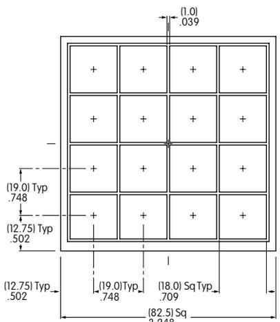
Insertable Legend Cards are supplied with the nonilluminated keypad assembly in Black, Gray and Yellow
