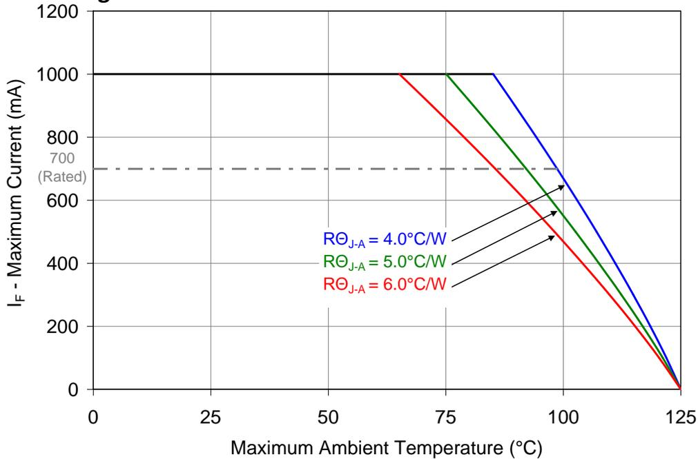
Figure 11: Maximum forward current vs. ambient temperature based on T<sub>J</sub>(MAX) = 125°C.
