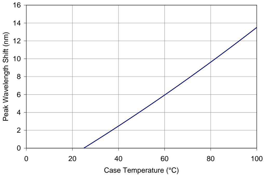
Figure 9: Typical peak wavelength shift vs. case temperature.
