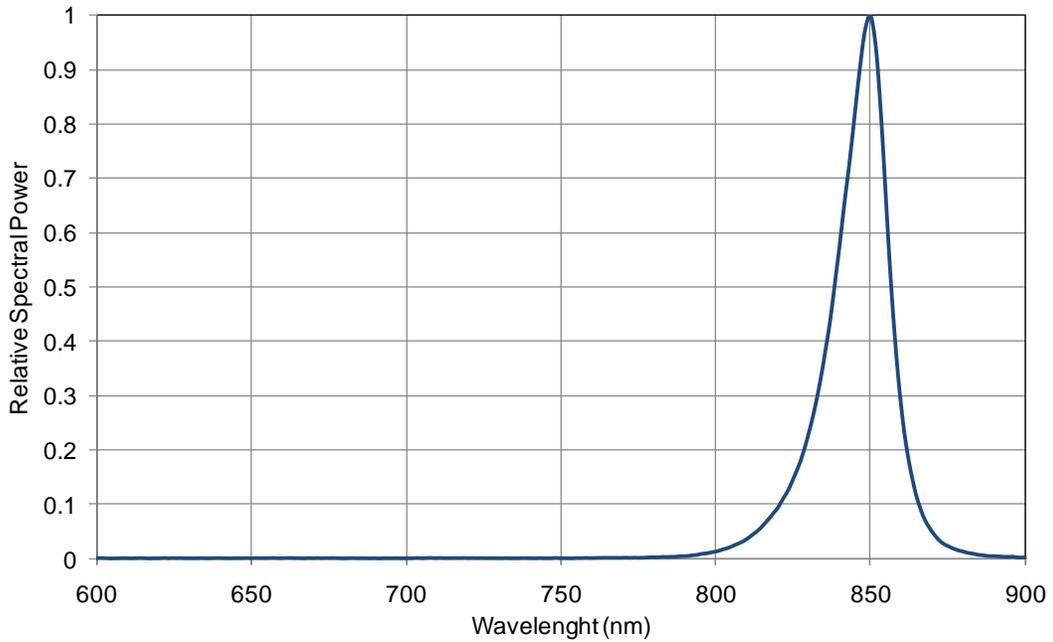
Figure 5: Relative spectral power vs. wavelength @ T<sub>c</sub> = 25°C.
