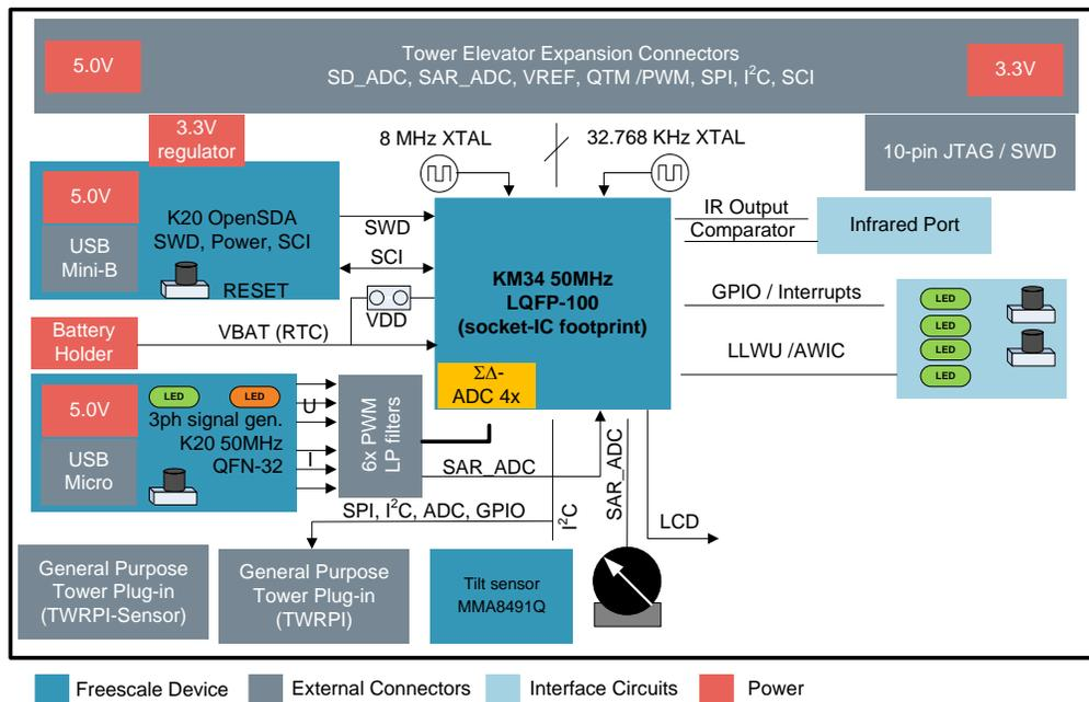
Figure 4. Block diagram of TWR-KM34Z50M tower board
