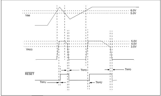
FIGURE 2-7: RESET Timing Diagram.
