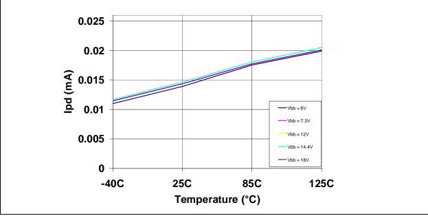
FIGURE 2-11: Typical I<sub>BBPD</sub> vs. Temperature.
