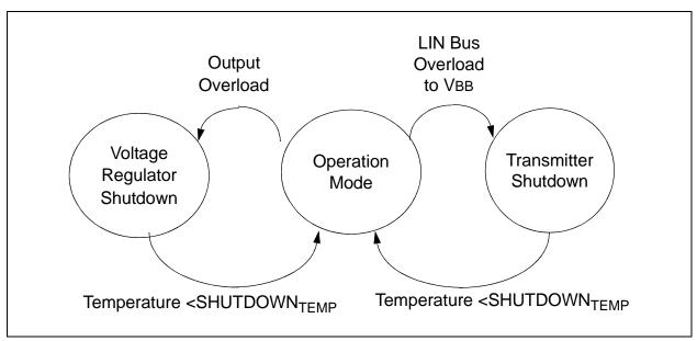
FIGURE 1-1: Thermal Shutdown State Diagrams.
