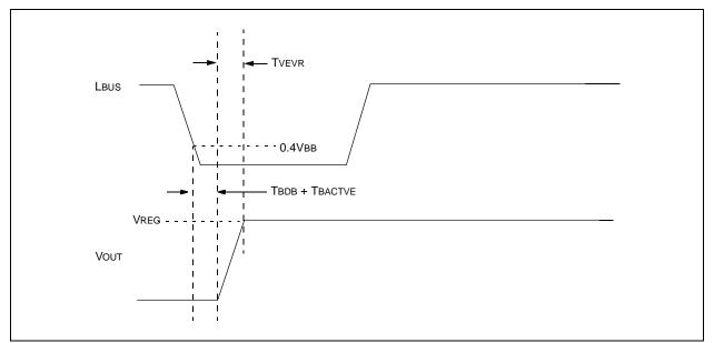
FIGURE 2-6: Regulator BUS WAKE Timing Diagram.
