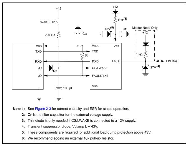
FIGURE 1-6: Typical MCP2021/MCP2021P Application.
