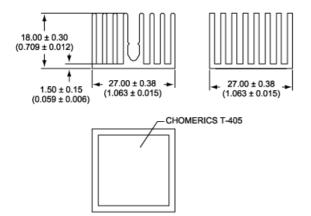
Width: 27.00 Length: 27.00 Height: 18.00 Base Thickness: 1.50 Fin Thickness: Length 1.63, Width 1.40 # of Fins: Length 8, Width 8 Fin Tip to Tip: 0.00 Finish: Black Anodize
