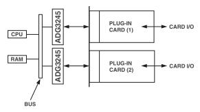
Figure 12. ADG3245 in a Hot Plug Application
