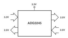
Figure 5. 3.3 V to 2.5 V Voltage Translation,  $\overline{SEL} = V_{CC}$  In this case, the output will be limited to 2.5 V, as shown in Figure 6.
