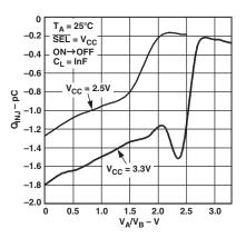
TPC 12. Charge Injection vs. Source Voltage
