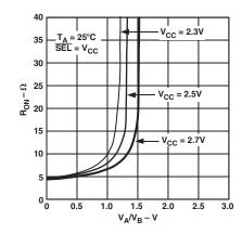
TPC 2. On Resistance vs. Input Voltage
