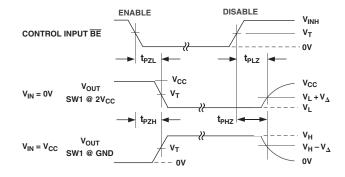
Figure 3. Enable and Disable Times
