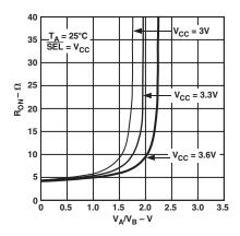
TPC 1. On Resistance vs. Input Voltage
