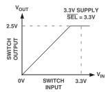
Figure 6. 3.3 V to 2.5 V Voltage Translation,  $\overline{SEL} = V_{CC}$ This device can be used for translation from 2.5 V to 3.3 V devices and also between two 3.3 V devices.
