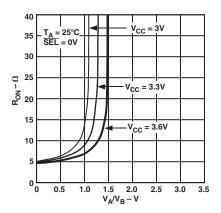
TPC 3. On Resistance vs. Input Voltage
