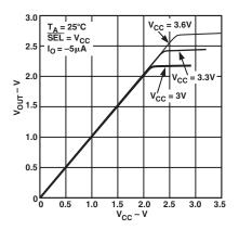
TPC 6. Pass Voltage vs.  $V_{CC}$
