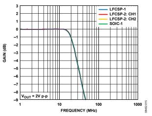
Figure 16. Large Signal Frequency Response for Various Packages
