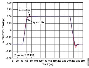
Figure 58. V<sub>OCM</sub> Large Signal Transient Response
