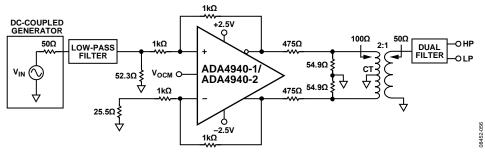
Figure 60. Test Circuit for Distortion Measurements
