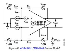
As with conventional op amp, the output noise voltage densities can be estimated by multiplying the input-referred terms at +IN and –IN by the appropriate output factor,
