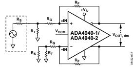
Figure 65. ADA4940-1/ADA4940-2 Configured for Unbalanced (Single-Ended) Input
