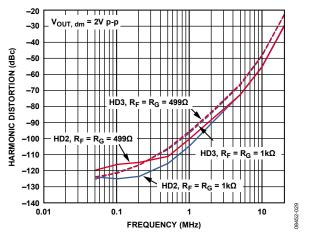
Figure 36. Harmonic Distortion vs. Frequency for Various R<sub>F</sub> and R<sub>G</sub> (LFCSP)
