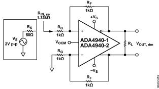
Figure 66. Calculating Single-Ended Input Impedance, R<sub>IN</sub>
