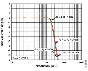
Figure 10. Large Signal Frequency Response for Various Gains and Loads
