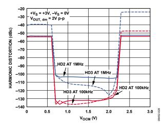
Figure 35. Harmonic Distortion vs. V<sub>OCM</sub> for 100 kHz and 1 MHz, 3 V Supply (LFCSP)
