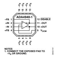
Figure 4. ADA4940-1 Pin Configuration (16-Lead LFCSP)
