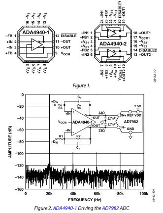
The ADA4940-1 is available in a Pb-free, 3 mm  $\times$  3 mm, 16-lead LFCSP, and an 8-lead SOIC. The ADA4940-2 is available in a Pb-free, 4 mm  $\times$  4 mm, 24-lead LFCSP. The pinout is optimized to facilitate printed circuit board (PCB) layout and minimize distortion. The ADA4940-1/ADA4940-2 are specified to operate over the -40°C to +125°C temperature range.
