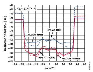
Figure 32. Harmonic Distortion vs. V<sub>OCM</sub> for 100 kHz and 1 MHz, ±2.5 V Supplies (LFCSP)
