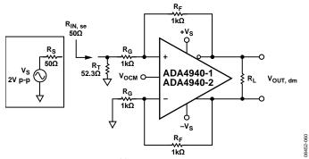
Figure 67. Adding Termination Resistor R<sub>T</sub>
