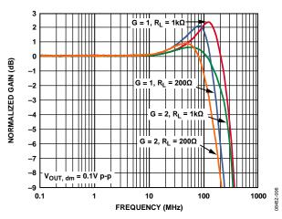
Figure 7. Small Signal Frequency Response for Various Gains and Loads (LFCSP)
