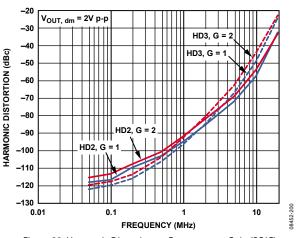
Figure 28. Harmonic Distortion vs. Frequency vs. Gain (SOIC)
