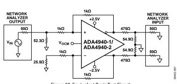
Figure 59. Equivalent Basic Test Circuit
