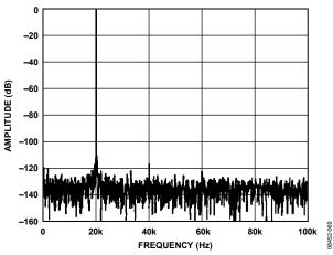
Figure 72. Distortion Measurement of a 20 kHz Input Tone (CN-0237)
