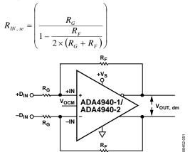
Figure 64. ADA4940-1/ADA4940-2 Configured for Balanced (Differential) Inputs
