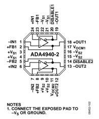
*Figure 6. ADA4940-2 Pin Configuration (24-Lead LFCSP)*
