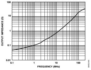
Figure 47. Closed-Loop Output Impedance Magnitude vs. Frequency, G = 1
