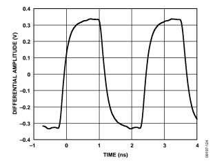
Figure 24. Output Waveform, LVDS (400 MHz)
