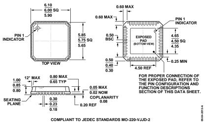
Figure 55. 40-Lead Lead Frame Chip Scale Package [LFCSP\_VQ] 6 mm × 6 mm Body, Very Thin Quad (CP-40-13) Dimensions shown in millimeters
