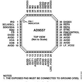
Figure 2. Pin Configuration
