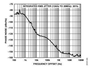
Figure 6. Absolute Phase Noise (Output Driver = HSTL),  $f_R = 19.44 \text{ MHz}$ ,  $f_O = 174.703 \text{ MHz}$ , DPLL Loop BW = 1 kHz,  $f_{SYS} = 49.152 \text{ MHz}$  Crystal
