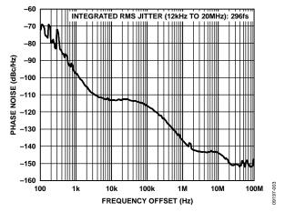
Figure 3. Absolute Phase Noise (Output Driver = HSTL),  $f_R = 19.44$  MHz,  $f_O = 622.08$  MHz, DPLL Loop BW = 50 Hz,  $f_{\rm SYS} = 49.152$  MHz Crystal
