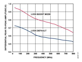
Figure 17. Amplitude vs. Toggle Rate, LVDS
