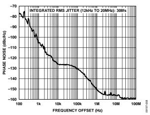
Figure 8. Absolute Phase Noise (Output Driver = HSTL),  $f_R = 2 \text{ kHz}$ ,  $f_O = 125 \text{ MHz}$ ,  $DPLL \ Loop \ BW = 100 \ Hz$ ,  $f_{SYS} = 49.152 \ MHz$  Crystal
