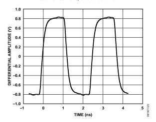
Figure 23. Output Waveform, HSTL (400 MHz)
