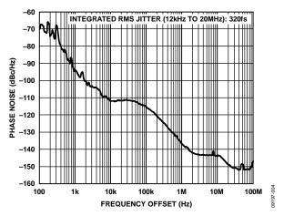
Figure 4. Absolute Phase Noise (Output Driver = HSTL),  $f_R = 19.44$  MHz,  $f_O = 644.53125$  MHz, DPLL Loop BW = 50 Hz,  $f_{SYS} = 49.152$  MHz Crystal
