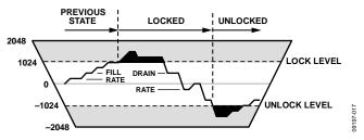
Figure 38. Lock Detector Diagram
