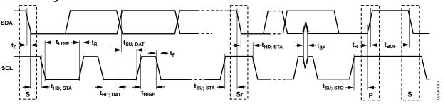
Figure 54. I<sup>2</sup>C Serial Port Timing
