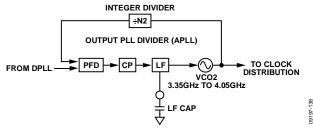
Figure 39. Output PLL Block Diagram
