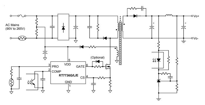
Figure 5. Application Circuit For RT7736G, RT7736L and RT7736E
