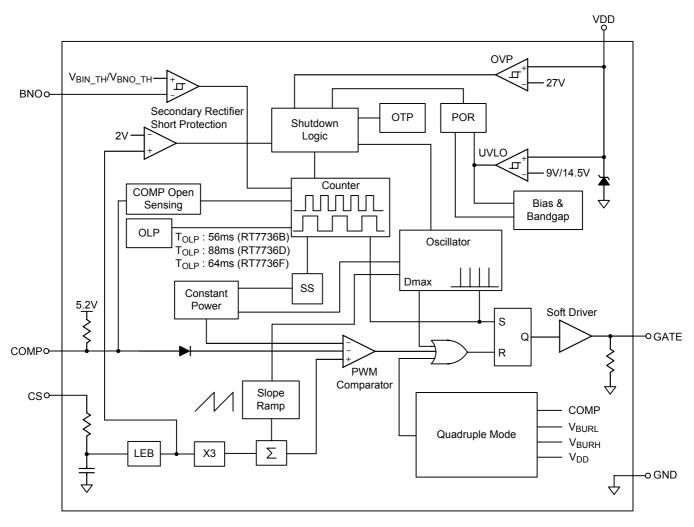
Figure 2. Block Diagram for RT7736B, RT7736D and RT7736F
