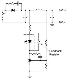
Figure 19. Feedback Resistor
