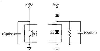
Figure 17. OVP for Output Voltage
