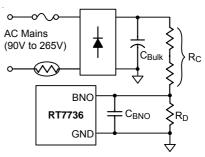
Figure 11. Brown-in/out Detected from Bulk Capacitor
