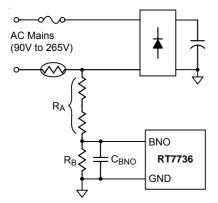
Figure 10. Brown-in/out Detected from AC Line Input
