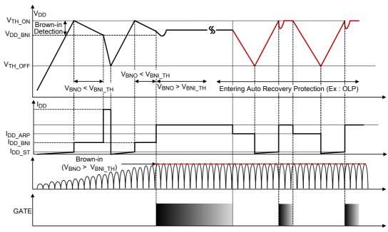
Figure 12. RT7736 Brown-in Detected Function
