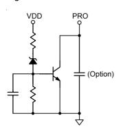
Figure 16. OVP for VDD
