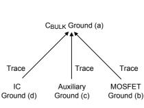
Figure 22. PCB Layout Guide
