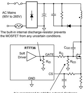
It is recommend to add the external dischargeresistor to avoid MOSFET false triggering.
