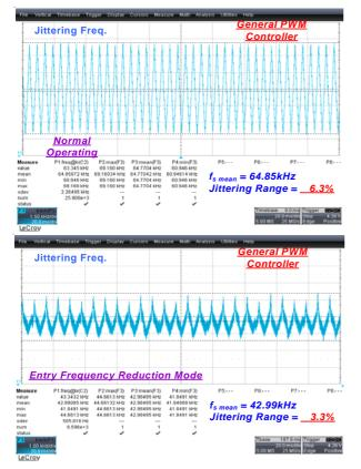
When the system enters frequency reduction mode, a output power relationship is formed between the feedback voltage  $V_{COMP}$  and the PWM switching frequency, and a new stable equilibrium point is eventually reached after back-and-forth adjustments. It limits the frequency jittering range is limited and the improving EMI function is poor, as shown in Figure 7.
