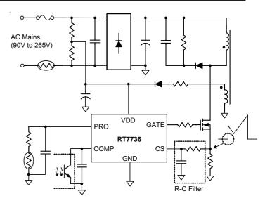
Figure 20. R-C Filter on CS Pin
