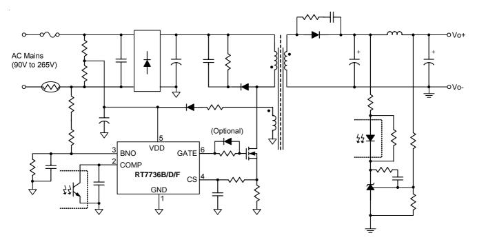
Figure 6. Application Circuit for RT7736B, RT7736D and RT7736F
