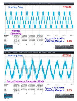
Figure 7. Frequency Jittering Range During Frequency Reduction Mode : General PWM Controller vs. RT7736
