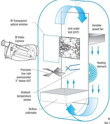
Figure 9. Vertical Wind Tunnel
