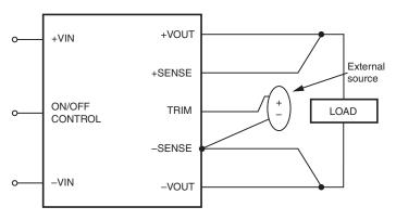
Figure 8. Trimming with an External Source
