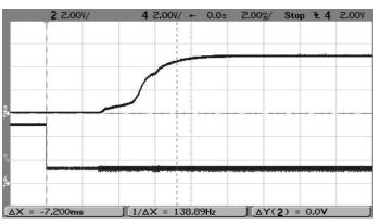
Enable Start-up (Vin=48V, lout=12A, Cload=1000uF, Ta=+25°C)
