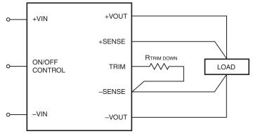
Figure 7. Trim Connections To Decrease Output Voltages
