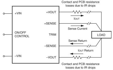
Figure 4. Remote Sense Circuit Configuration
