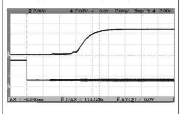
Enable Start-up (Vin=48V, lout=0A, Ta=+25°C) Trace 2=0utput, Trace 4= Enable.
