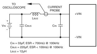
Figure 2. Measuring Input Ripple Current
