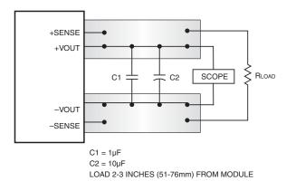
Figure 3. Measuring Output Ripple/Noise (PARD)
