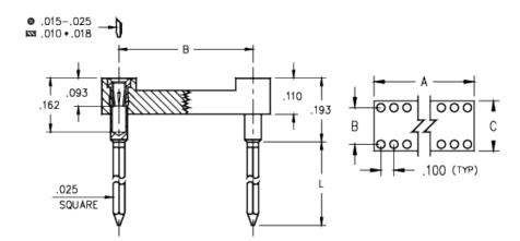
**Description:** DIP Dual In Line Socket Wire-Wrap Tail Open Frame **Plating Code:** Shell Plating: 200 μ" Tin (matte finish) over 100 µ" Nickel Inner Contact Plating: 30 μ" Gold over 50 μ" Nickel Packaging: Packaged in Tubes
