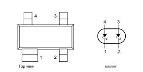
Fig.1 Simplified outline (SOT143B), pin configuration and symbol.
