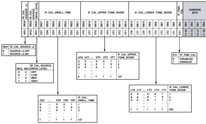
Figure 68. Register 6—IF Fine Calibration Setup Register Map
