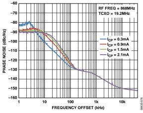
Figure 12. Phase Noise Response at 868 MHz,  $V_{DD} = 2.3 V$
