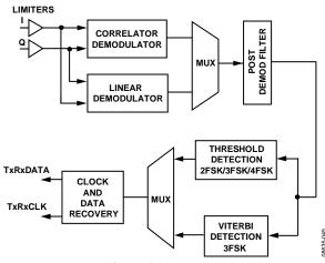
Figure 46. Overview of Demodulation, Detection, and CDR Process
