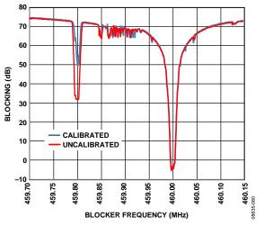
Figure 27. Image Rejection, Uncalibrated vs. Calibrated
