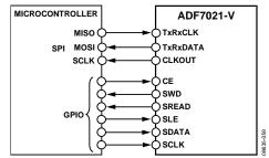
Figure 60. ADF7021-V (SPI Mode) to Microcontroller Interface
