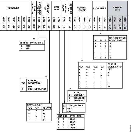
Figure 63. Register 1—Oscillator Register Map
