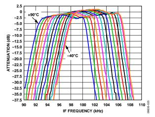
Figure 28. Variation of IF Filter Response with Temperature (IF\_FILTER\_BW = 9 kHz, Temperature Range Is  $-40^{\circ}$ C to  $+90^{\circ}$ C in 10° Steps)
