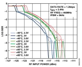
Figure 22. 2FSK Sensitivity vs. VDD and Temperature at 460 MHz
