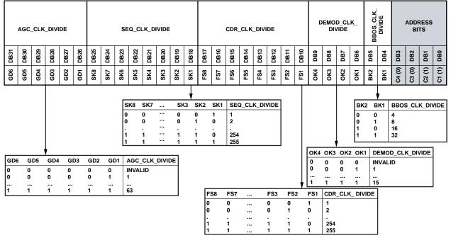
Figure 65. Register 3—Transmit/Receive Clock Register Map
