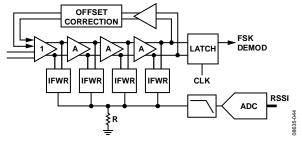
Figure 45. RSSI Block Diagram
