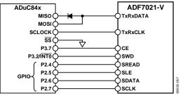
Figure 58. ADuC84x to ADF7021-V Connection Diagram
