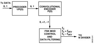
Figure 42. 3FSK Encoding
