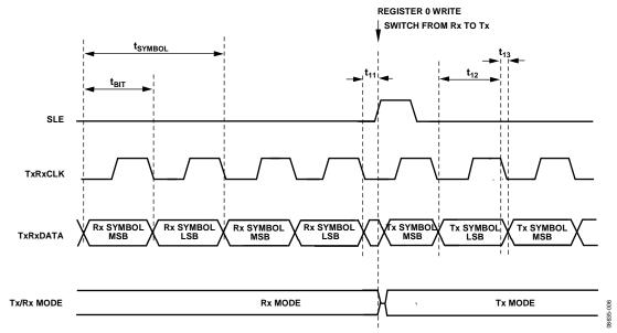
Figure 6. Receive-to-Transmit Timing Diagram in 4FSK Mode
