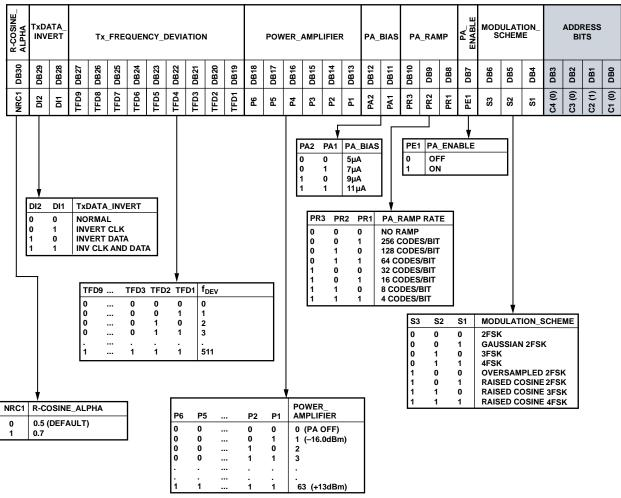
Figure 64. Register 2—Transmit Modulation Register Map
