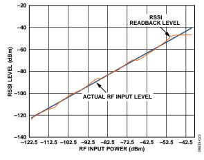
Figure 26. Digital RSSI Readback Linearity
