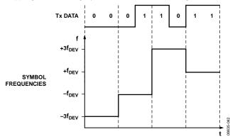
Figure 43. 4FSK Bit-to-Symbol Mapping
