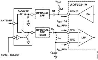
Figure 50. ADF7021-V with External Tx/Rx Switch
