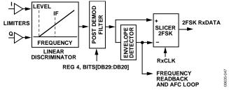
Figure 48. Block Diagram of Linear FSK Demodulator
