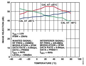
Figure 52. Image Rejection vs. Temperature After Initial Calibrations  $at -40^{\circ}$ C, +25°C, and +85°C
