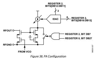
The PA is equipped with overvoltage protection, which makes it robust in severe mismatch conditions. Depending on the application, users can design a matching network for the PA to exhibit optimum efficiency at the desired radiated output power level for a wide range of antennas, such as loop or monopole antennas. See the LNA/PA Matching section for more information.
