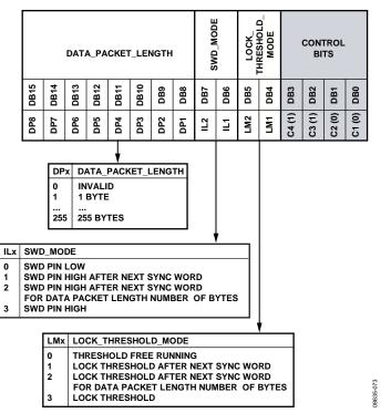
Figure 74. Register 12—SWD/Threshold Setup Register Map
