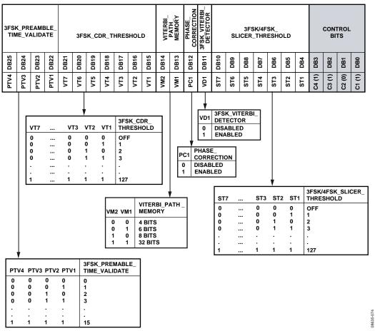
Figure 75. Register 13—3FSK/4FSK Demodulation Register Map
