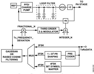
Figure 40. Transmit Modulation Implementation
