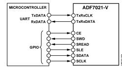
Figure 59. ADF7021-V (UART Mode) to Asynchronous Microcontroller Interface
