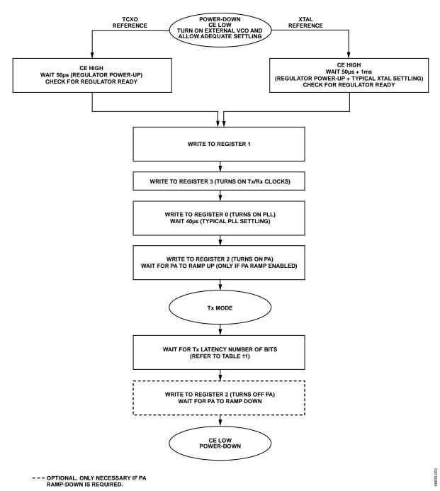
Figure 54. Power-Up Sequence for Transmit Mode
