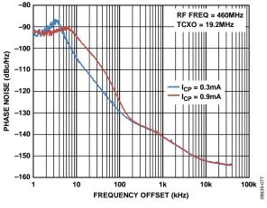
Figure 11. Phase Noise Response at 460 MHz,  $V_{DD} = 3 V$
