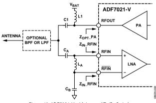
Figure 49. ADF7021-V with Internal Tx/Rx Switch
