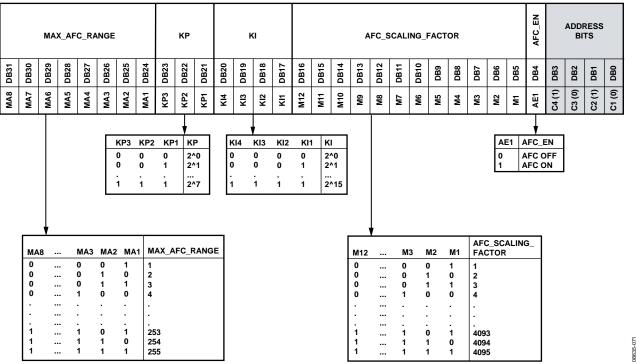
Figure 72. Register 10—AFC Register Map
