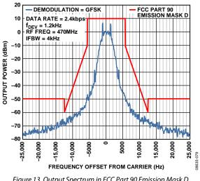
Figure 13. Output Spectrum in FCC Part 90 Emission Mask D and GFSK Modes
