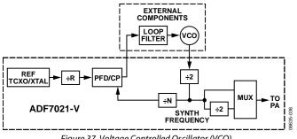
Figure 37. Voltage Controlled Oscillator (VCO)
