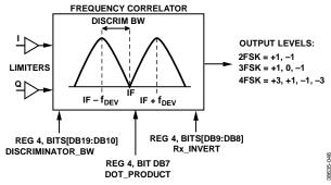
Figure 47. 2FSK Correlator FSK Demodulator Operation
