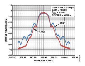
Figure 16. Output Spectrum in 2FSK and GFSK Modes
