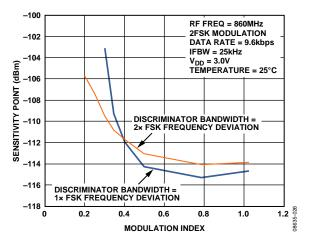
Figure 29. 2FSK Sensitivity vs. Modulation Index and Correlator Discriminator Bandwidth
