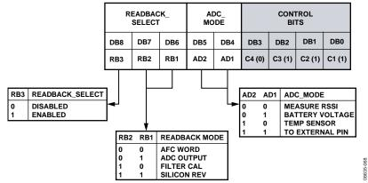
Figure 69. Register 7—Readback Setup Register Map
