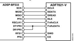
Figure 61. ADSP-BF533 to ADF7021-V Connection Diagram
