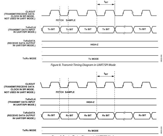
Figure 9. Receive Timing Diagram in UART/SPI Mode
